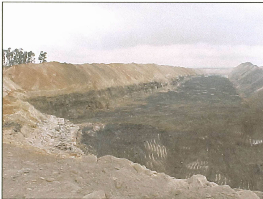
Figure 8-6. A 60 m wide cut at the opencast pit at Kromdraai.
