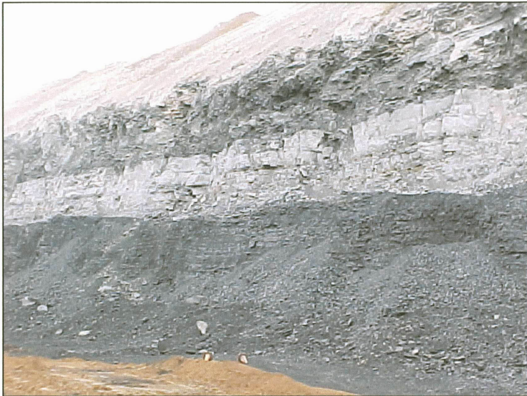
Figure 8-3. The No. 2 Seam in relation to the overlying strata in the opencast pit at Kromdraai Colliery.
