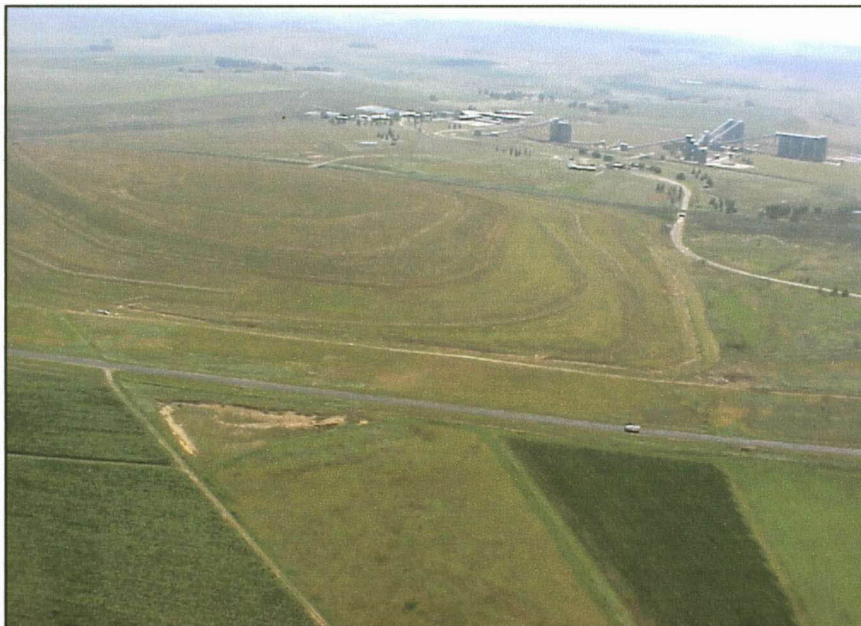
Figure 4-3. Rehabilitated discard dump with N17 road in forefront and mine buildings in the background (Photo: Chris Naudé - Ingwe Coal).
