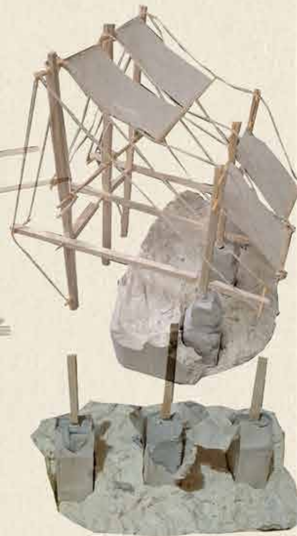
Figure 5.18: Construction touchstone showing the temporality of its structure by being able to assemble and disassemble it Also showing foundations that will stay behind on site when the timber structure is removed (author, 2024)
