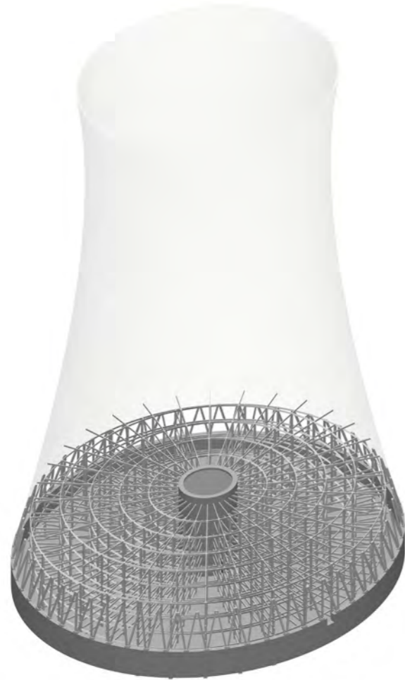
EXISTING COOLING TOWER STRUCTURE WALLS + INTERNAL STRUCTURE
