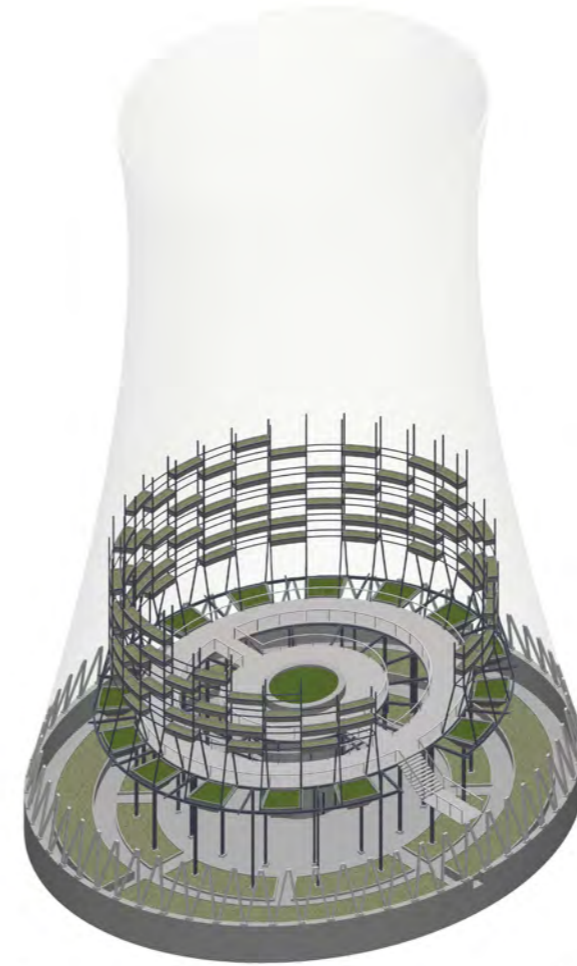
ADDING MODULAR STEEL STRUCTURE WITH PLANTERS TO ACCOMMODATE CREEPER PLANTS
