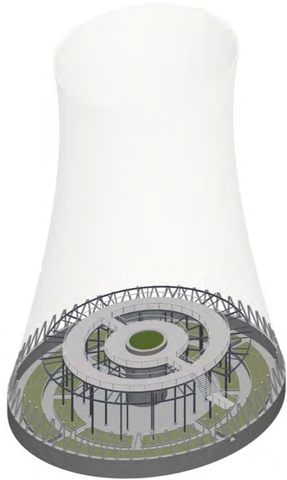
REPLACING DENSE INTERNAL STRUCTURE WITH STEEL STRUCTURE TO ACCOMMODATE WALKWAY + ADDING PLANTERS ON GROUND LEVEL
