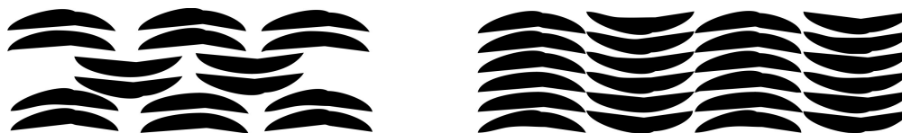
Figure 2.26. Schematic representation of stacking possibility for banana shaped liquid crystals.
