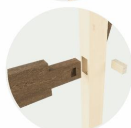
ADAPTED AHIKATAME BEAM JOINT (TENSION)
