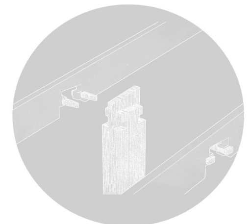
ADAPTED ASHIKATAME JOINT (USED IN TENSION)
