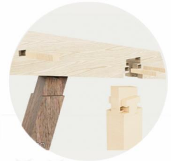
ADAPTED ASHIKATAME RAFTER JOINT (TENSION)
