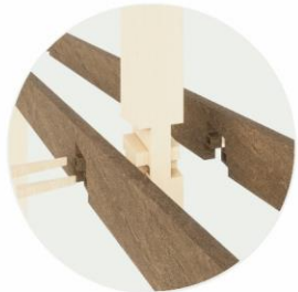
ADAPTED AHIKATAME BEAM JOINT (TENSION)
