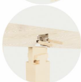
ADAPTED ASHIKATAME JOINT (TENSION)
