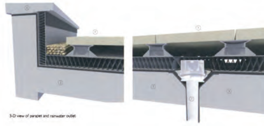
3-D view of parapet and rainwater outlet
