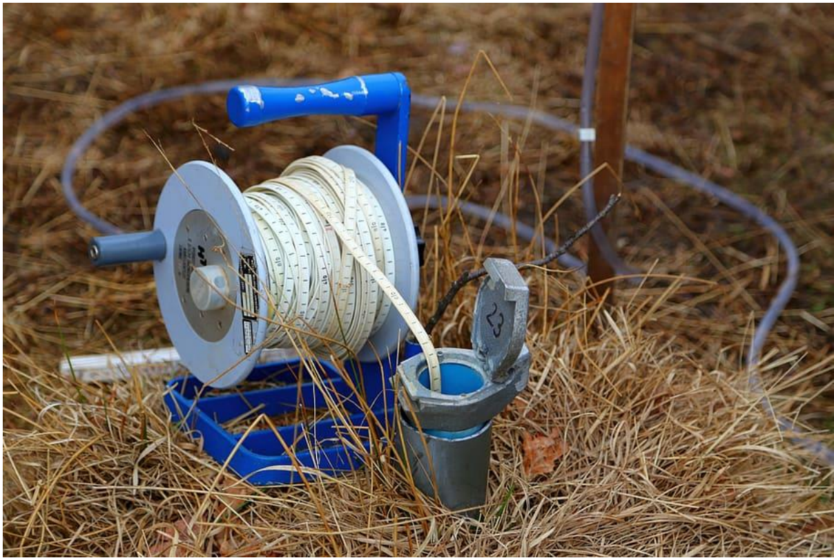
Figure 3-3: Picture showing groundwater level measurements from a monitoring borehole (Wallpaper Flare, 2022)
