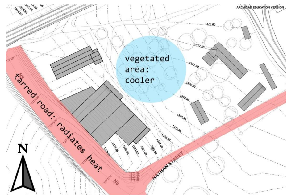
Figure 5.3: Utilising the site in a more sustainable manner identifying cooler and warmer spaces (Author, 2019).
