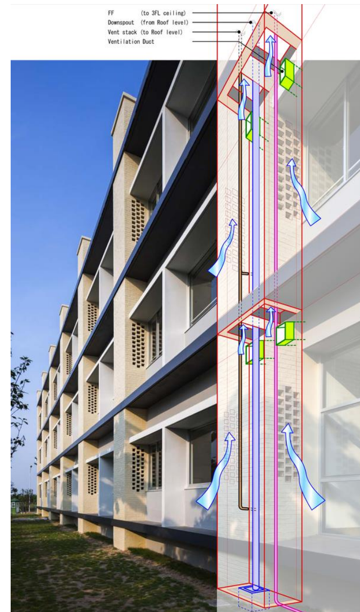
Figure 5.9; Air inlets incorporated into the building. (Taisei design planner architects and engineers, 2017: Online).
