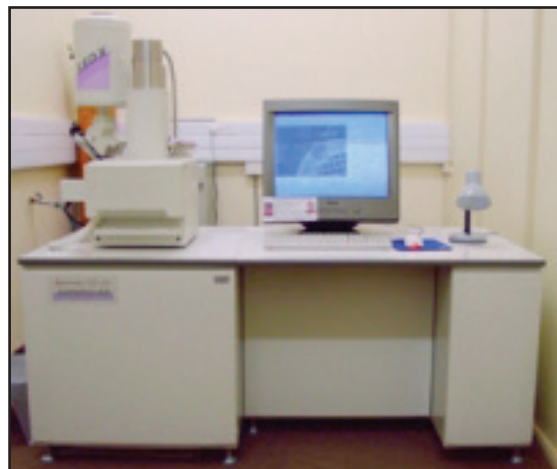
Figure 2.3 The SEM at the Centre of Microscopy at the University of the Free State, South Africa. This instrument is of the type Shimadzu SSX550 (UFS, 2011).
