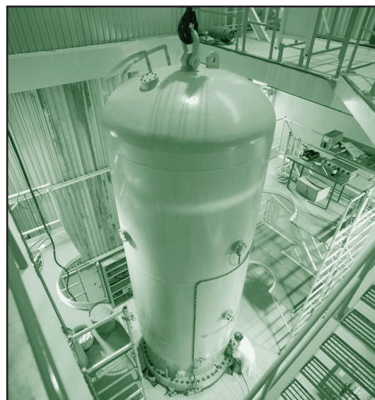
Figure 2.6 Van der Graaf accelerator as the one used for the beam generation. (EU, 2012).
