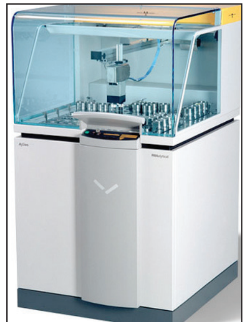
Figure 2.9 A PANalytical WD-XRF Axios spectrometer as the one used in the Department of Geology at the University of the Free State, South Africa. (ETH, 2011).
