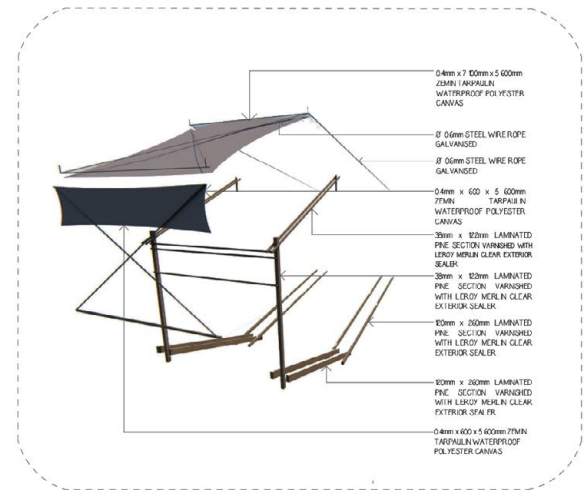
DETAIL 01A103 - SKELETAL SCREENING DEVICE NTS
