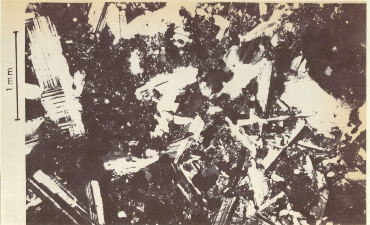
FIGURE 10.16a Relict igneous texture in metadolerite from the Nariams area. The pyroxenes are largely replaced by hornblende.
