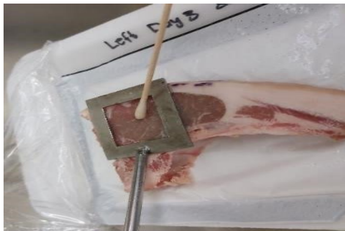
Fig. 3.4. Sterile template placed on chop, swab samples taken within the 2.5 X 2.5 cm 2 area.
