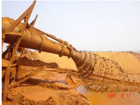
Figure 2.5: A photograph of a cyclone in action. Cyclones are used for backfilling the post-mined areas with sand.
