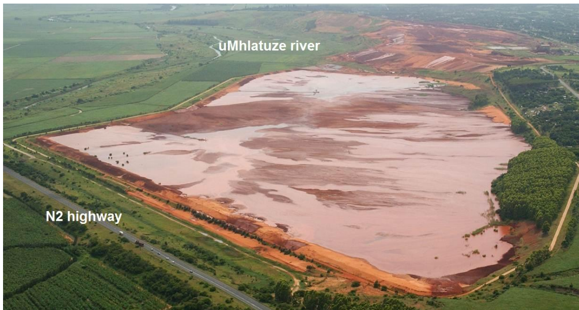
Figure 2.3: The residue storage facility (RSF) which contains slimes (slit and clay). The RSF covers an area of about 130 ha.
