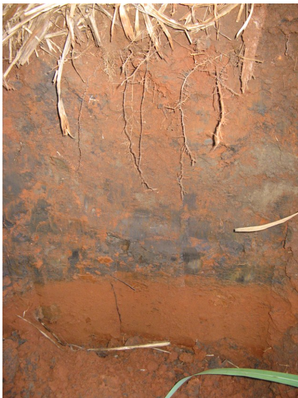
Figure 4.1: A typical profile of disturbed soil to a depth of \pm 100 cm in the unmined area.
