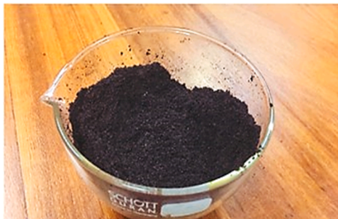
Fig. 2. Graphene oxide powder obtained by Hummer's method of preparation.
