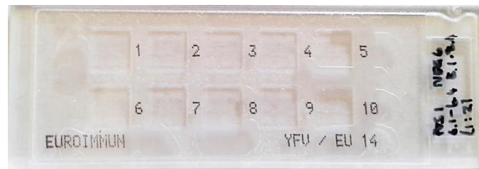
Figure 3.2: Illustration of an anti-YFV biochip slide for the detection of antibodies directed against YFV
