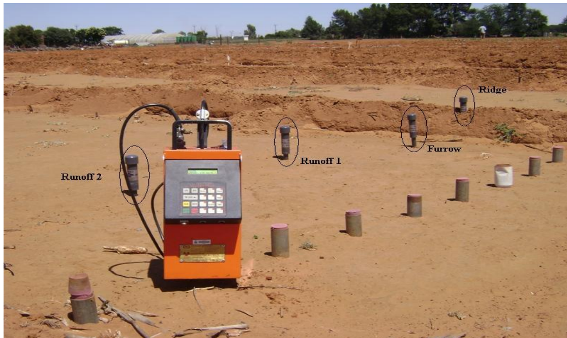
Figure 5.2 DFMA probes installed at different sections of the micro-landscape created by IRWH.
