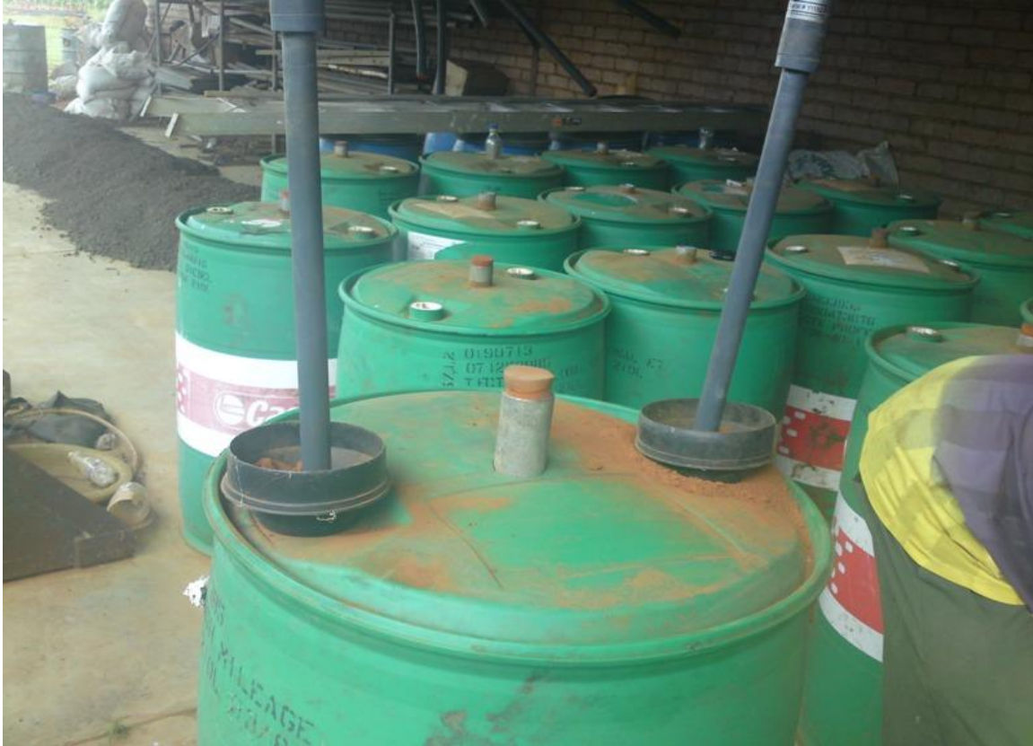
Figure 4.4 Two 1200 mm DFM probes inserted into a soil filled drum for calibration.
