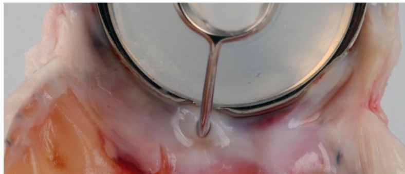
FIGURE 4.58: Pannus overgrowth can be seen at the junction between the proximal strut, valve housing and the pericardial patch.
