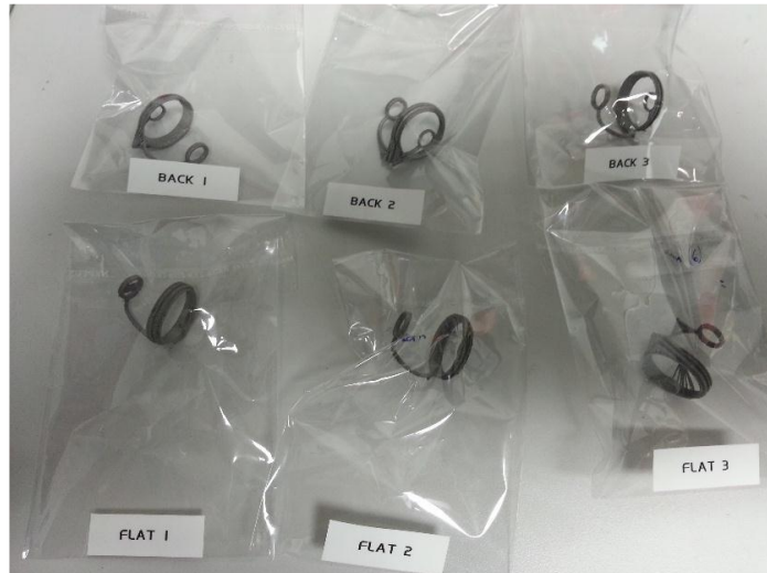
FIGURE 3: Samples of the titanium housing in the two orientations Flat and Back. The assemblies have been cleaned and the supportive material removed.
