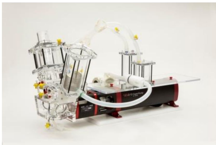
FIGURE 3.10: The ViVibro pulse duplicator (Adapted from www.vivitolabs.com )
