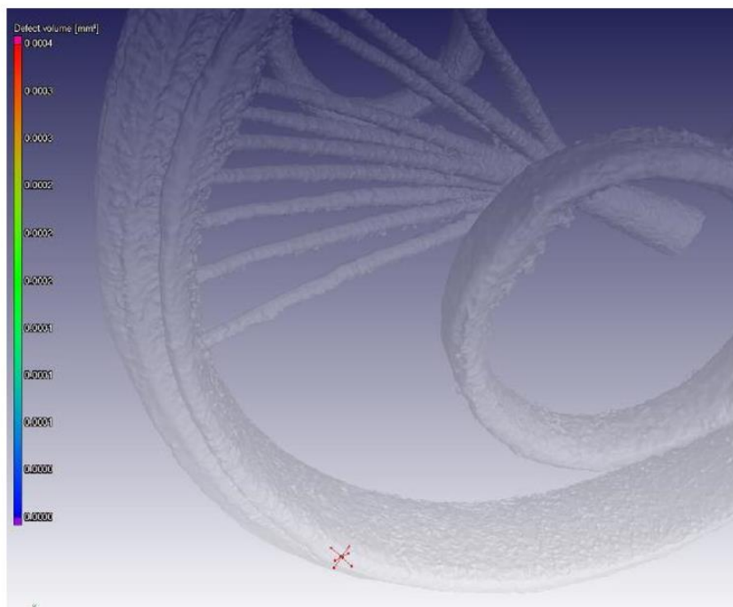
FIGURE 4: Computed tomography of Flat 2 with a 120 micron pore indicated by the red cross on the housing.
