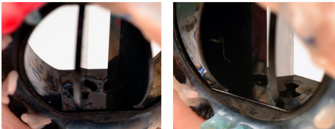
FIGURE 4.34: The hinge mechanism of the Carbomedics valve from different angles viewed from the PA.
