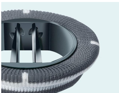
FIGURE 2.16: The Carbomedics valve showing the hinge mechanism. Leaflets rotate in the two semi-circular leaflet hinge depressions. Both the leaflets and the housing is covered with pyrolytic carbon and the dacron sewing cuff is impregnated with silver nitrate to reduce the incidence of Infective endocarditis. (Adapted from www.surgicaltechnology.com/15-149-CS-Page3-.html )
