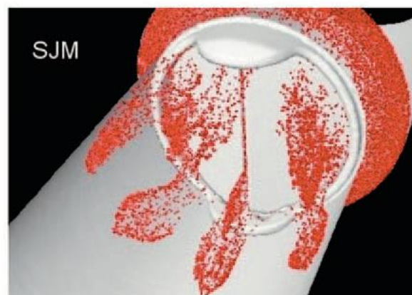
FIGURE 2.22: Particle dispersion patterns during the closed or leakage phase of an SJM bi-leaflet valve (Adapted from Dumont et al. , 2007).
