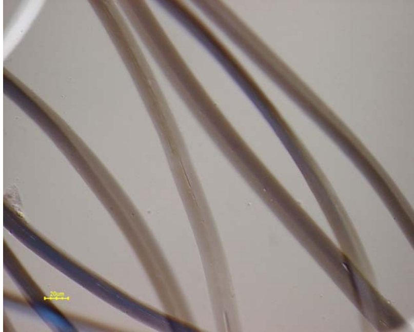
Photo 5: The longitudinal view of the acrylic Courtelle fibre as seen under a light microscope.
