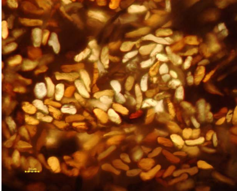
Photo 2(a): The cross-sectional view of the Gonometta postica silk as seen under a light microscope.
