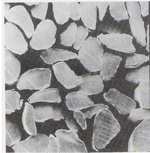
The cross-sectional view of silk (Kadolph, 2001).
