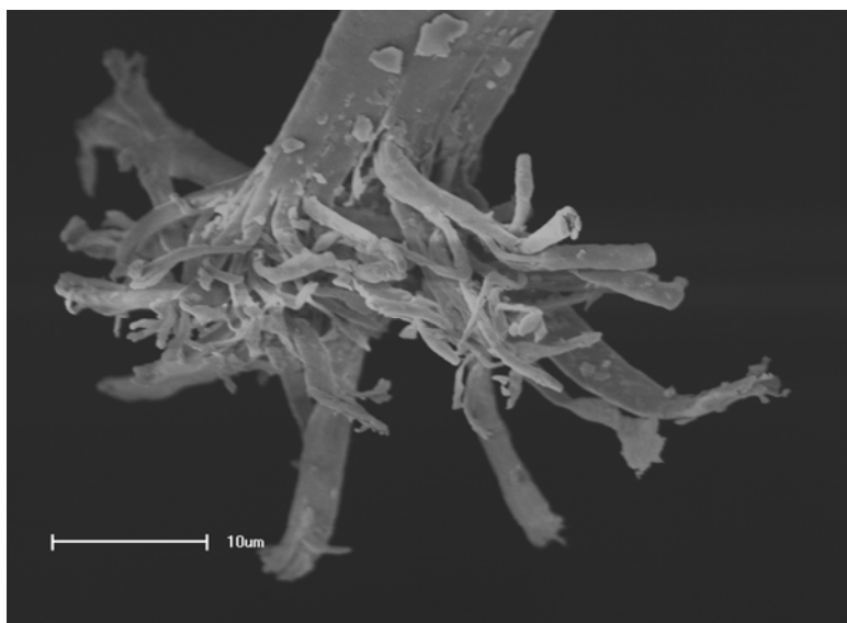
Photo 7(d): A scanning electron micrograph of a broken Gonometta postica silk fibre end showing the fibrillar structure.
