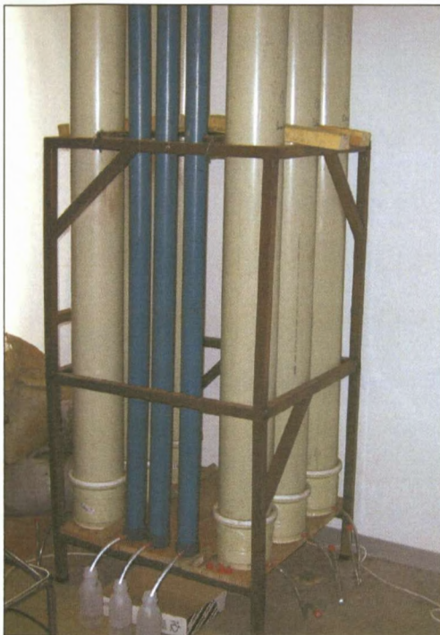
Figure 6-31: Photograph of the leaching columns.
