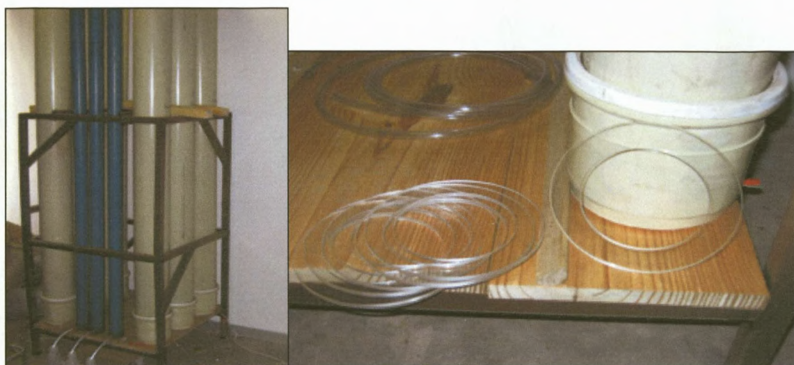
Figure 5-8: Photograph of the different leaching columns used (left) and annular rings (right).
