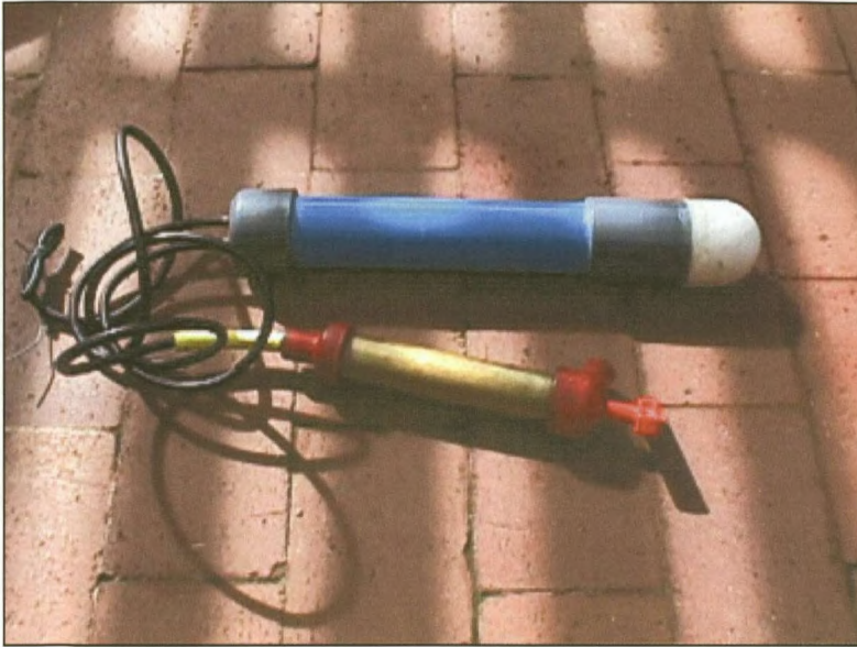
Figure 5-6: Porous cup lysimeters and vacuum pump.
