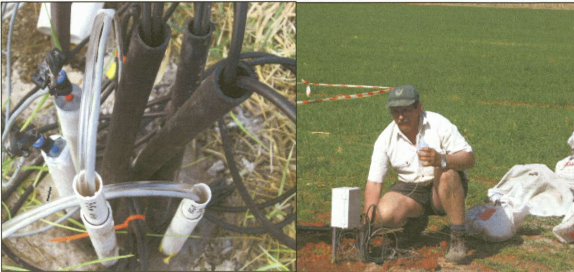
Figure 5-7: Installation of tensiometers (left) and replenishment (right).
