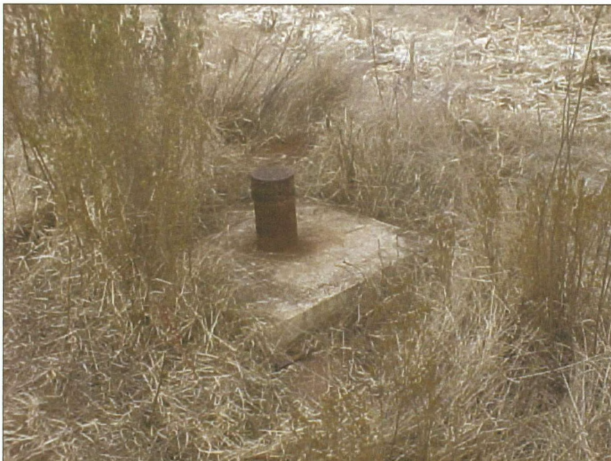
Figure 6-1: Monitoring borehole at Kleinkopje Pivot 4.
