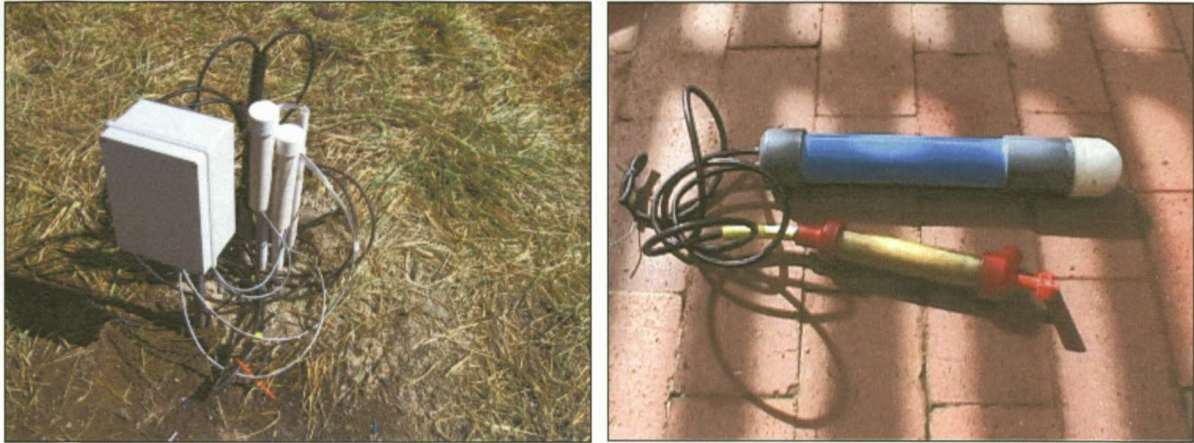
Figure 6-16: The porous cup and tensiometer installation (left) and porous cup sampler plus vacuum pump (right).
