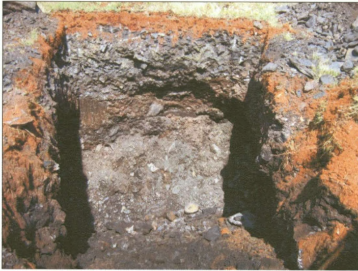
Figure 7-38: Pit in the spoils, illustrating the heterogeneity of the spoils.
