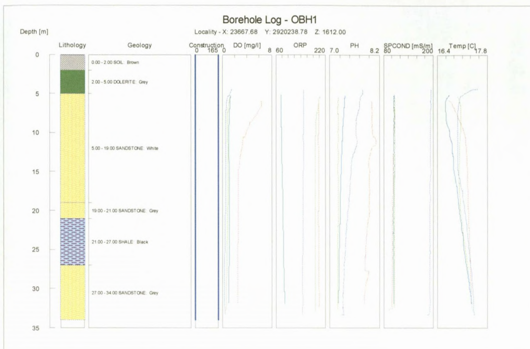
Figure 3-25: Multi-parameter profiling of OBH1.
