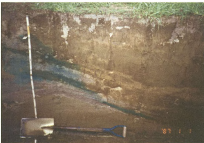
Figure 4-11: Funnel flow at field site. Blue dye flowing vertically (unsaturated flow) moves laterally when it encounters a sloping coarse-texture lens. (Source: Soil and Water Lab Website, Cornell University).
