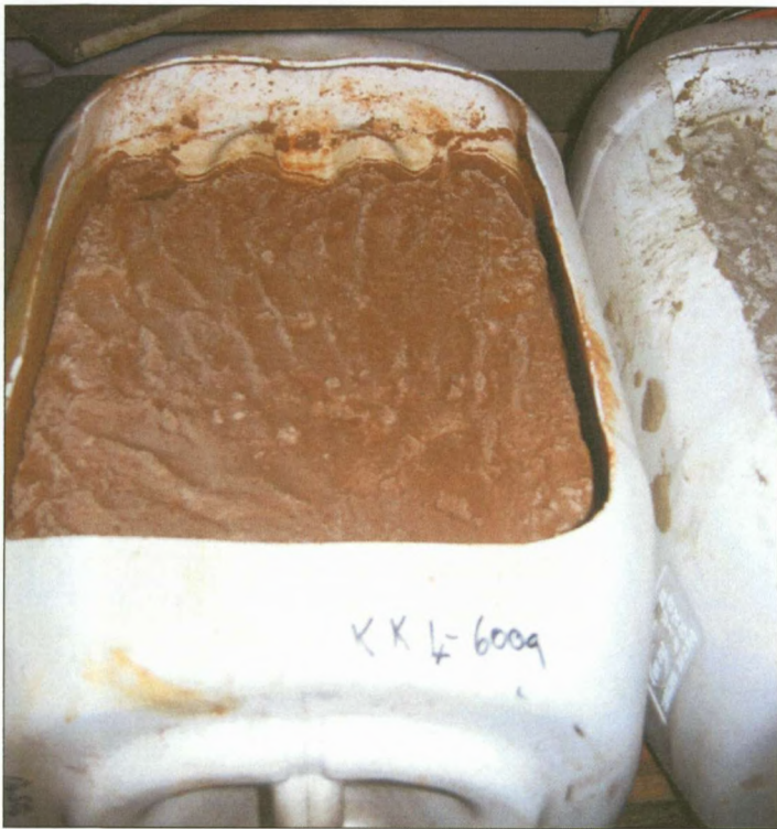
Figure 6-42: Leaching drums with different types of soils and gypsum concentrations.
