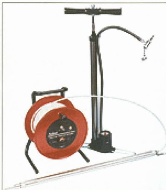
Figure 5-4: Specific Depth Sampler (from www.solinst.com )
