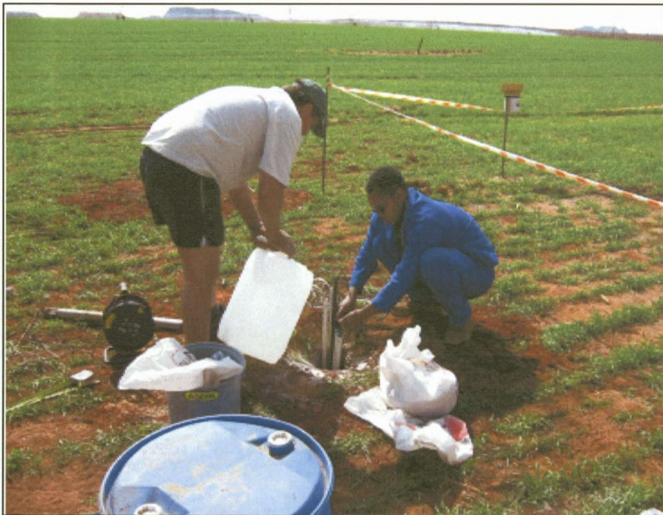
Figure 6-17: Porous cup installation at Pivot 4.
