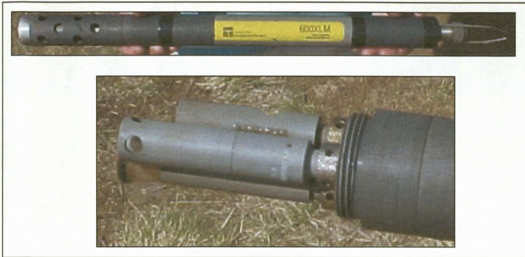
Figure 5-1: Multi-parameter probe with different sensors.
