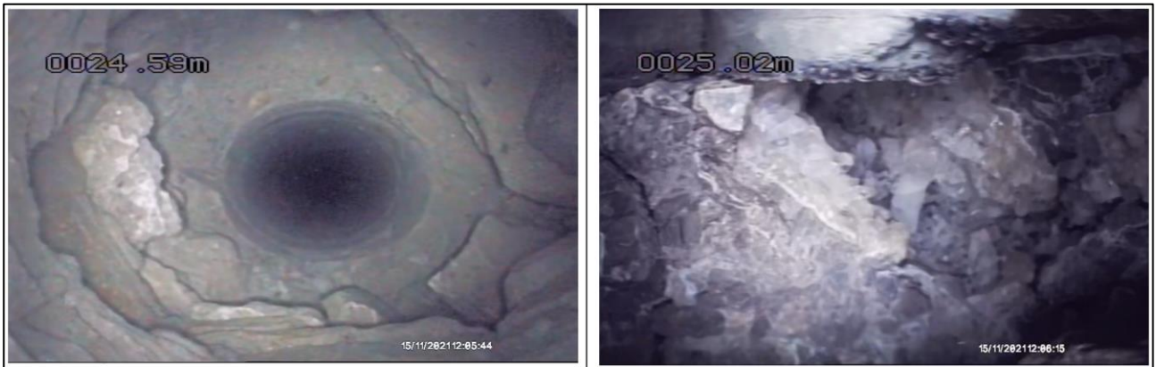
Figure 38: Fractured zone intersected with quartz growth in the fracture openings
