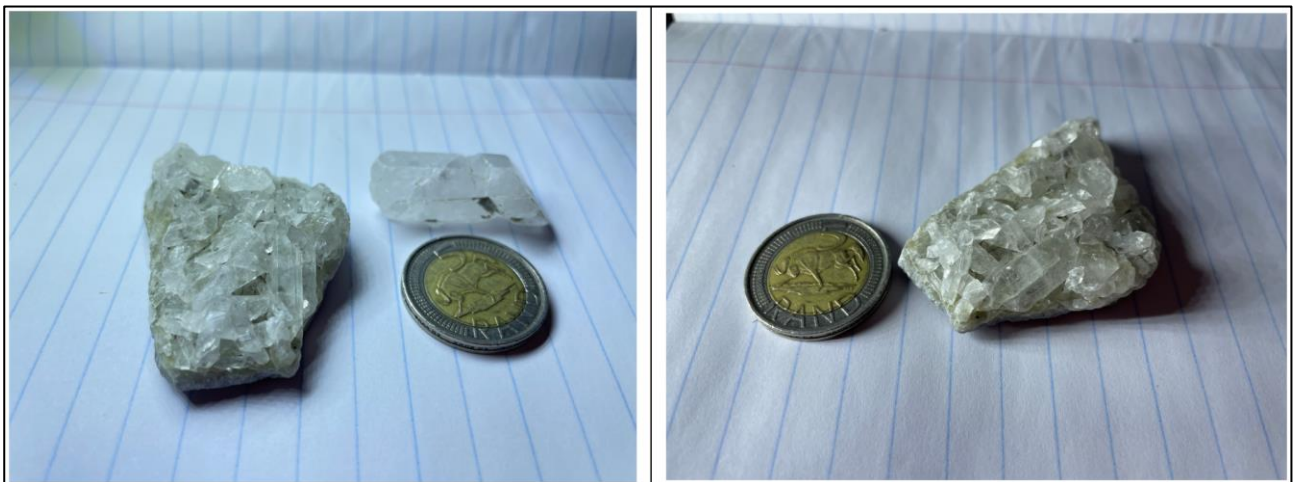
Figure 39: Quartz crystals on fractured zone drill chips from the drilling of borehole SL11
