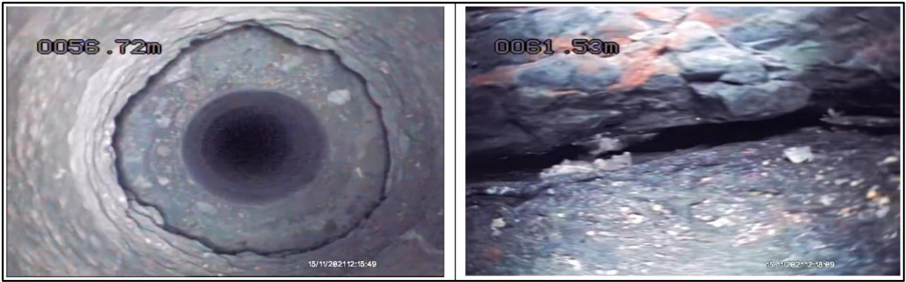
Figure 37: Screenshots of large open fractures in borehole SL11. Left: down-hole view of a fracture at 56.72 m, right: a side view of a fracture at 61.53 m
