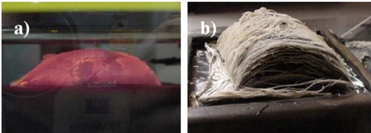
Figure 2.12 Images of (a) flax twill weave in a cone calorimeter, and (b) a burnt flax unidirectional fabric sample. Reprinted from [138], Copyright 2012, with permission from Elsevier
