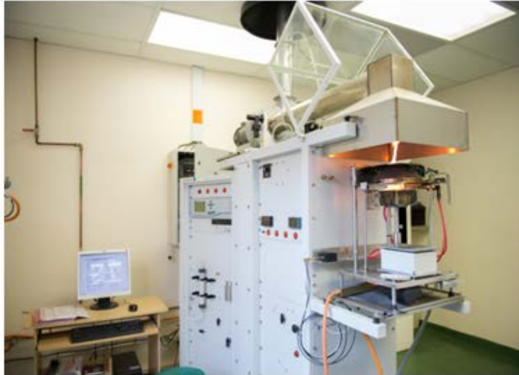
Figure 2.3 Cone calorimeter apparatus (from the Council for Scientific and Industrial Research (CSIR) fire testing laboratory)
