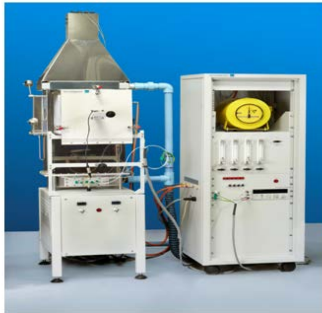
Figure 2.8 Ohio State University heat release (OSU) apparatus. Reprinted from [126], with permission from Fire Testing Technology Limited
