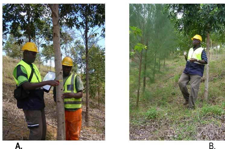
Figure 3.6 Instruments used to measure DBH and height. A. Diameter tape used for DBH measurements. B. Vertex hypsometer used for height measurements.
