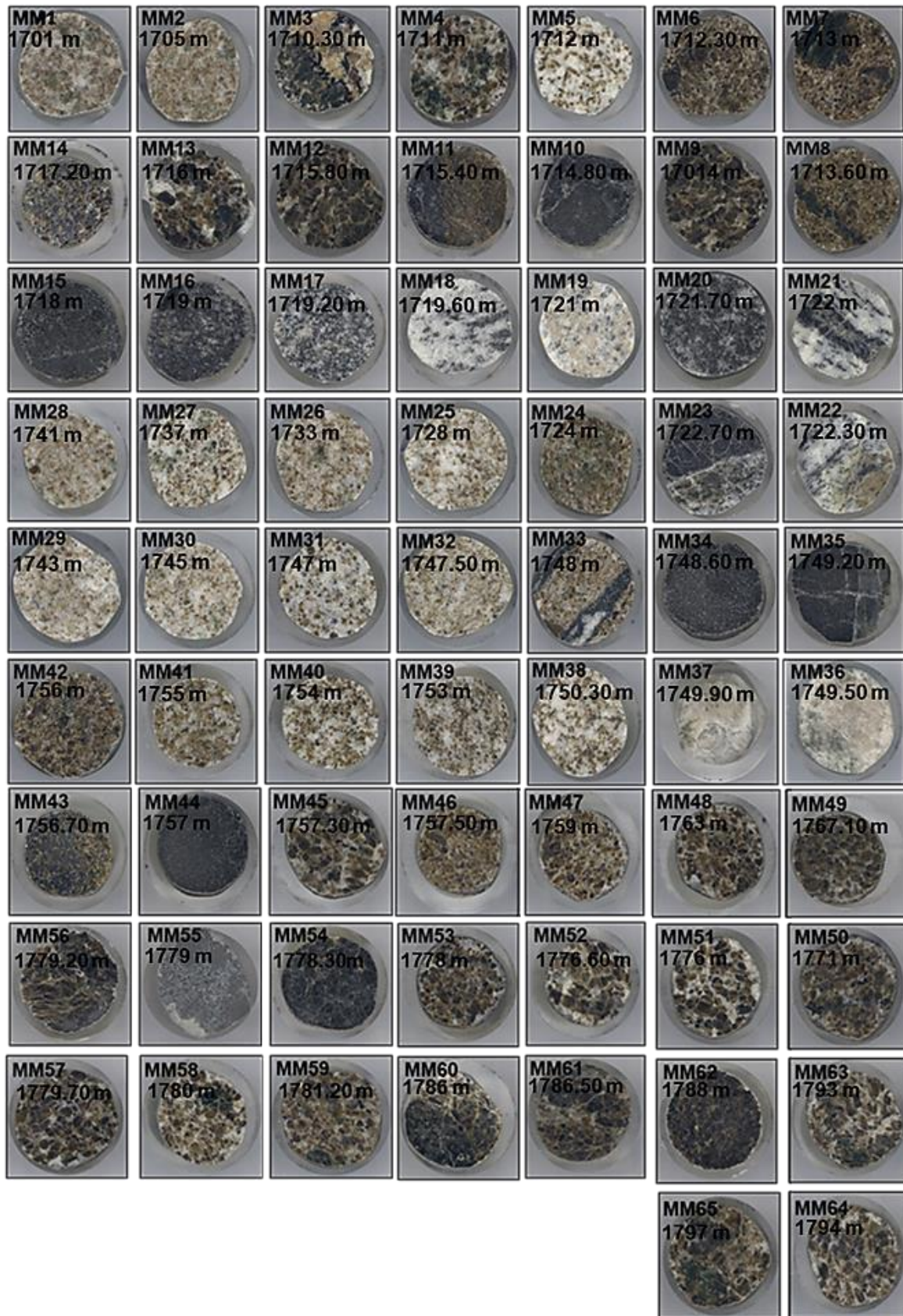
Figure 7: Polished blocks prepared from BH7929.
