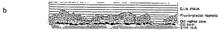
Schematic section, not to scale, showing the various lithostratigraphic components in connection with the aquifer.
