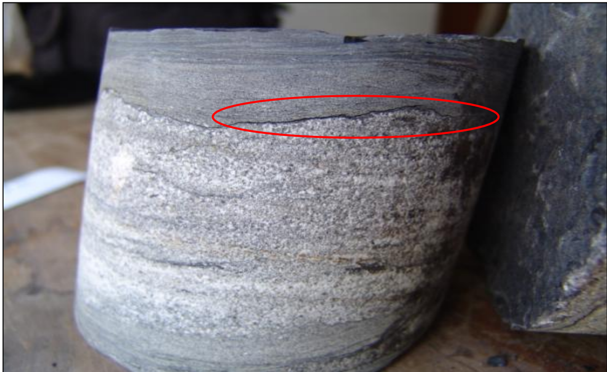
Figure 90: Rocks from the fractured aquifer zone, showing a bedding plane fracture outlined in red.
