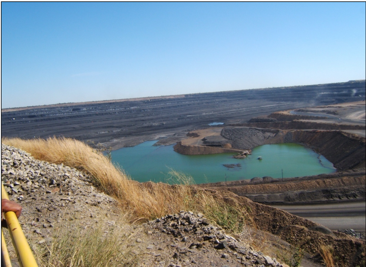
Figure 158: Surface runoff and groundwater inflow concentrated in a single location in the mine workings, courtesy of the Grootegeluk mine.
