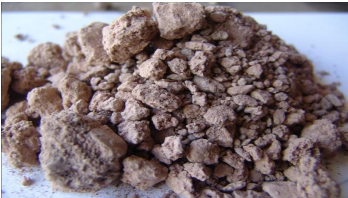
Figure 71: Sample GGSVZ1.4 4 m below the surface with acid potential.
