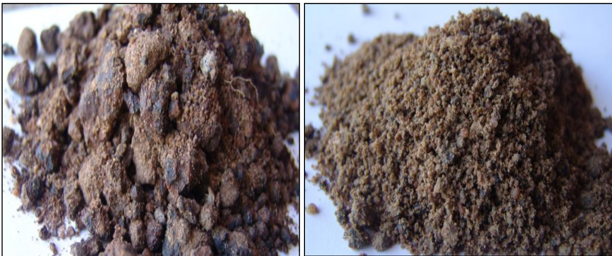
Figure 69: Sample GT3.2 (on the left) with acid potential and sample GT3.3 (on the right) with no acid potential
