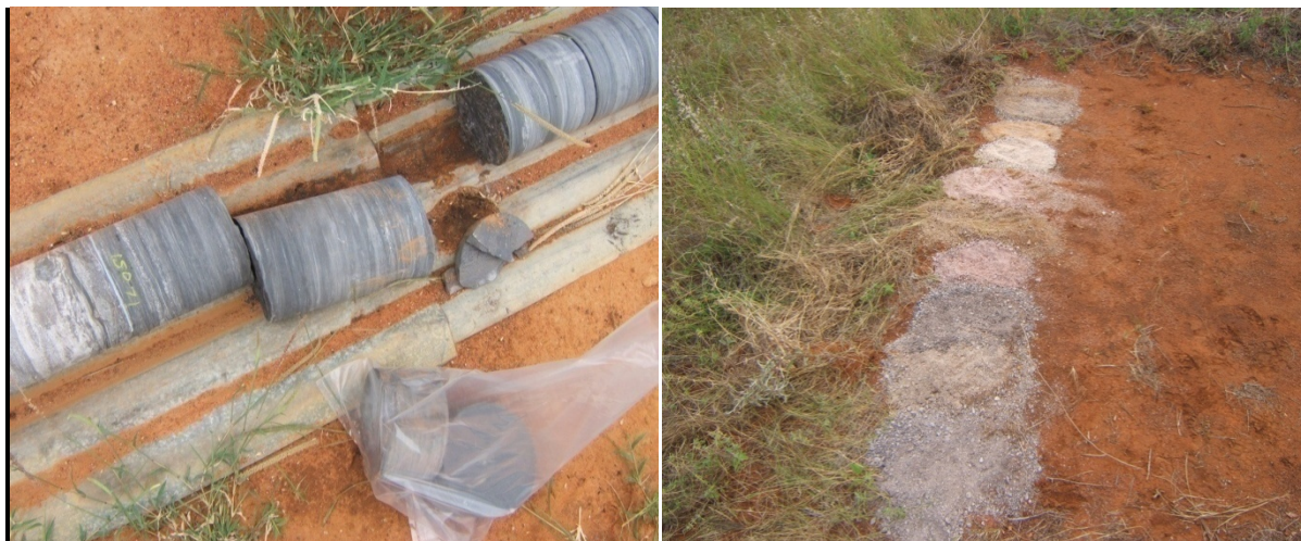
Figure 28: To the left Core samples, to the right Chip samples.
