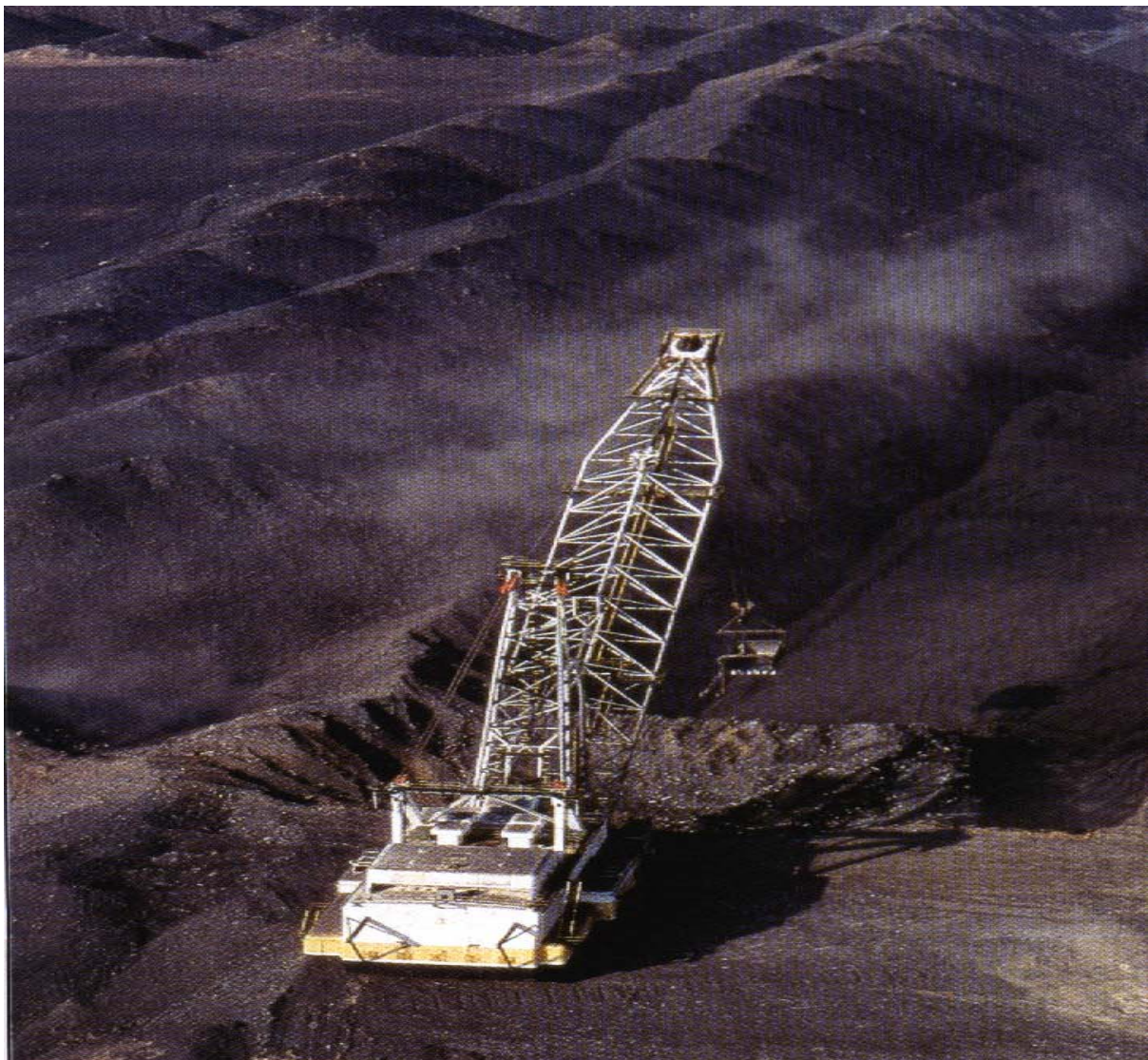
Figure 2: Dragline mining in an opencast pit (from Snyman, 1998, Optimum Colliery).
