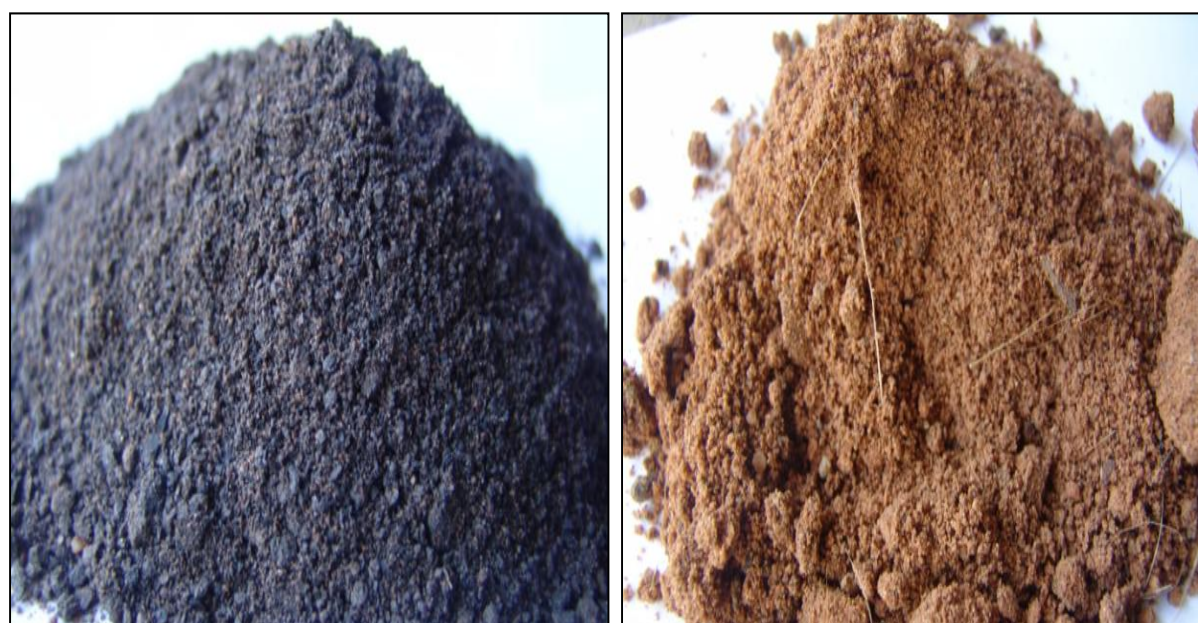
Figure 67: Samples GT1.9 & GT7.1, respectively, with acid potential.
