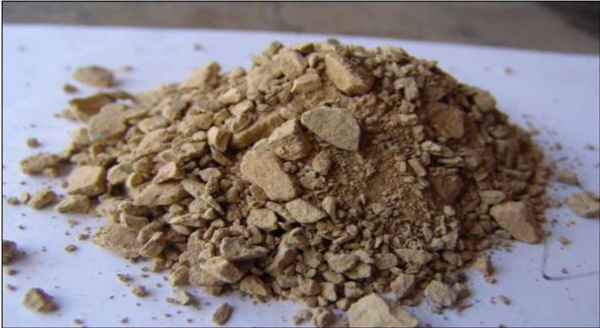
Figure 70: Sample GGVZ1, collected 1 m below the surface with acid potential.
