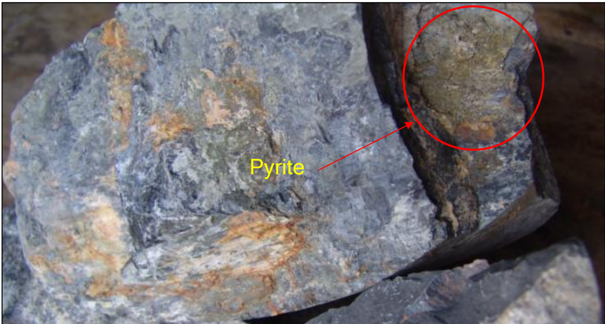
Figure 65: Sample SS6 showing the presence of pyrite.
