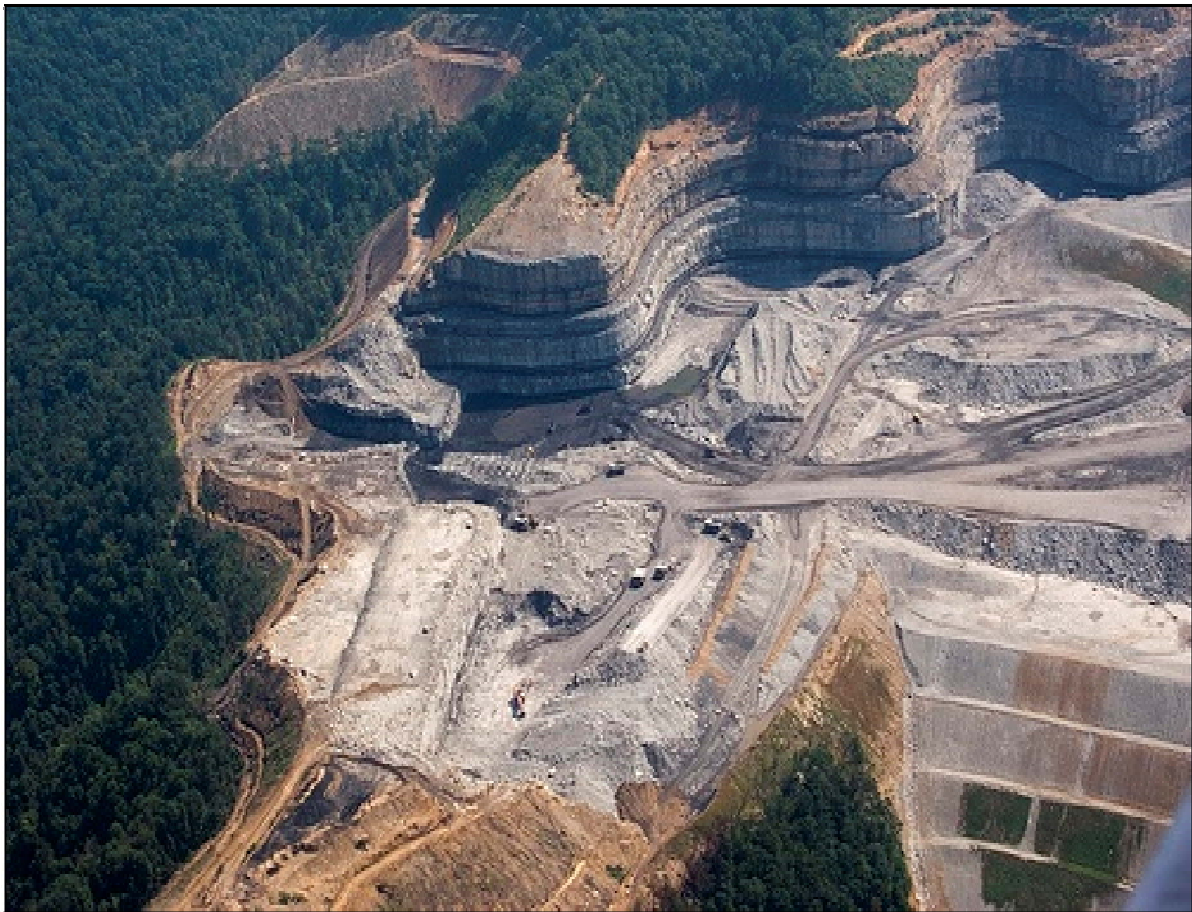
Figure 5: Mountaintop removal mining (www.coal-is-dirty.com).
