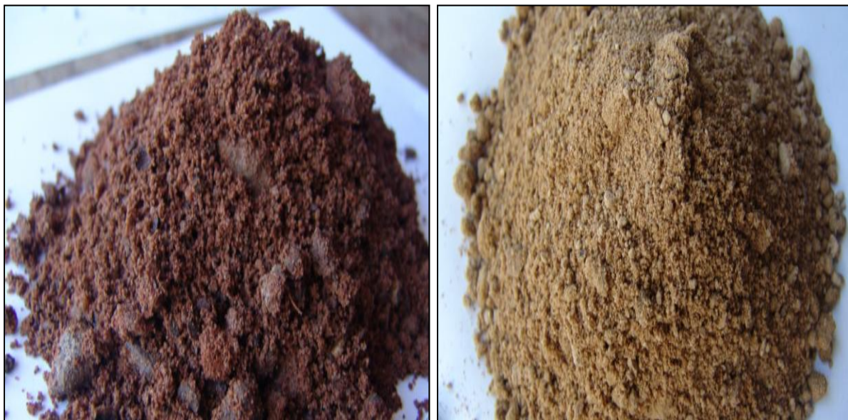
Figure 66: Samples GT1.1 & GT7.5, respectively, with no acid potential.
