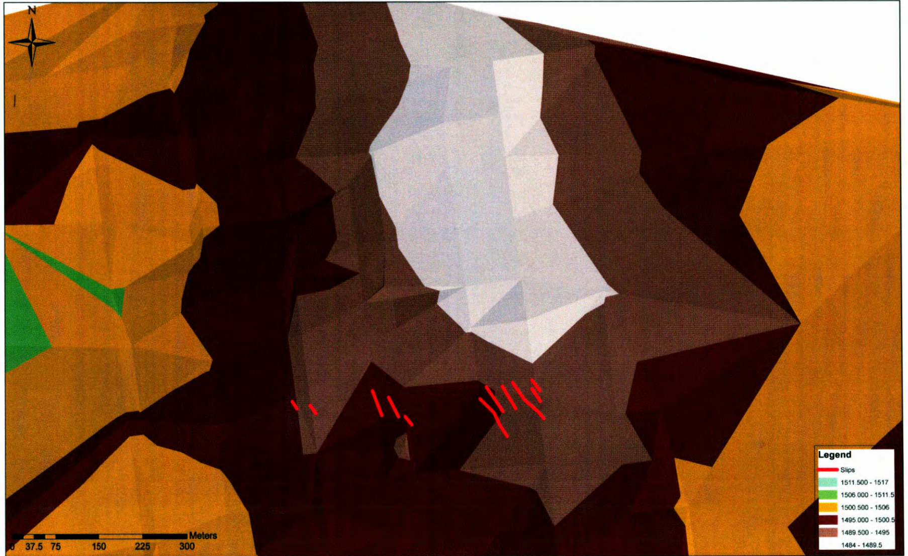
Figure 20: Slip zone 1 at Matla Coal Ltd. No. 2 Mine associated with the palaeo topography.
