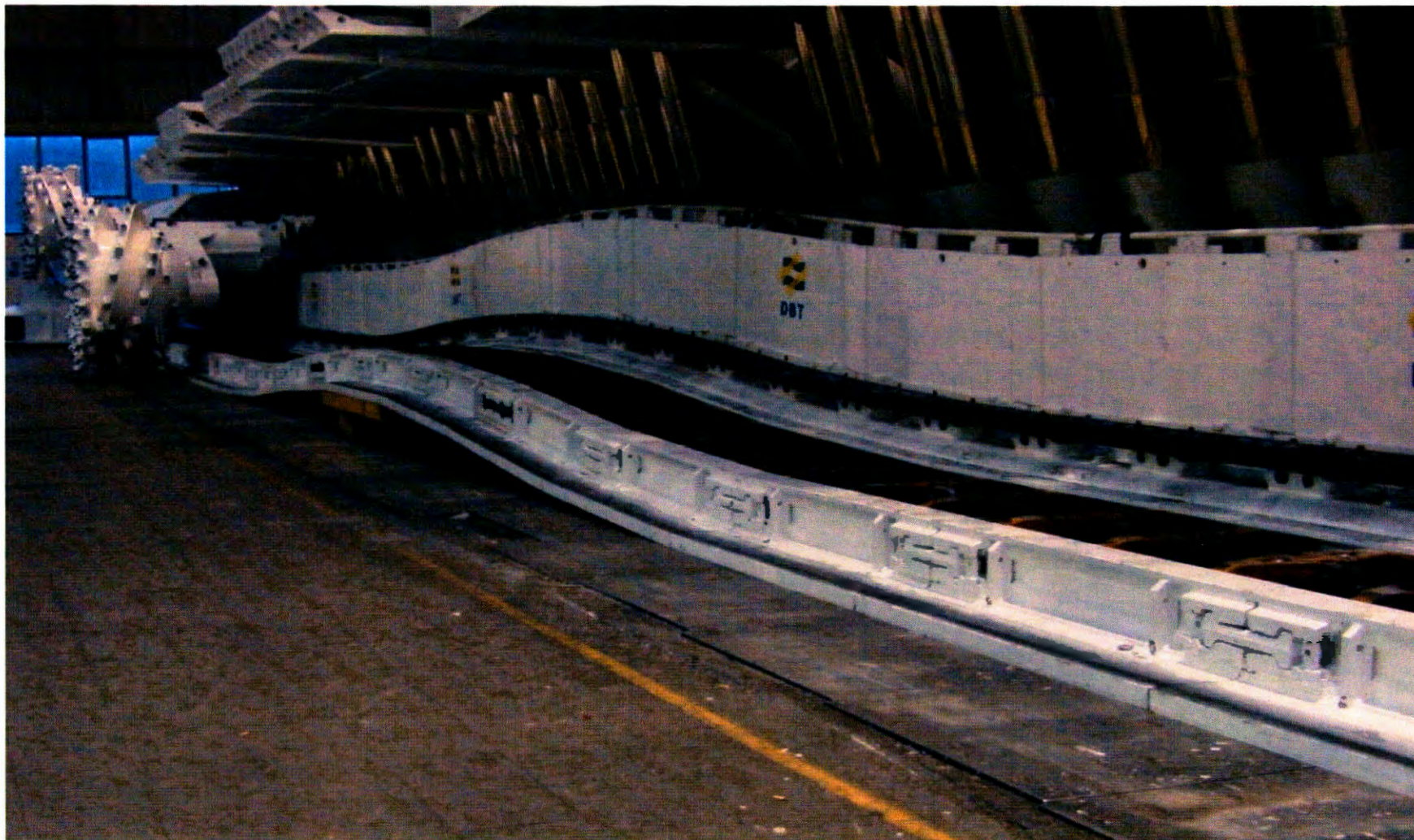
Figure 35: AFC (Automatic Face Conveyor) used in the coal cutting operation at Matla Coal Ltd No. 2 Mine.
