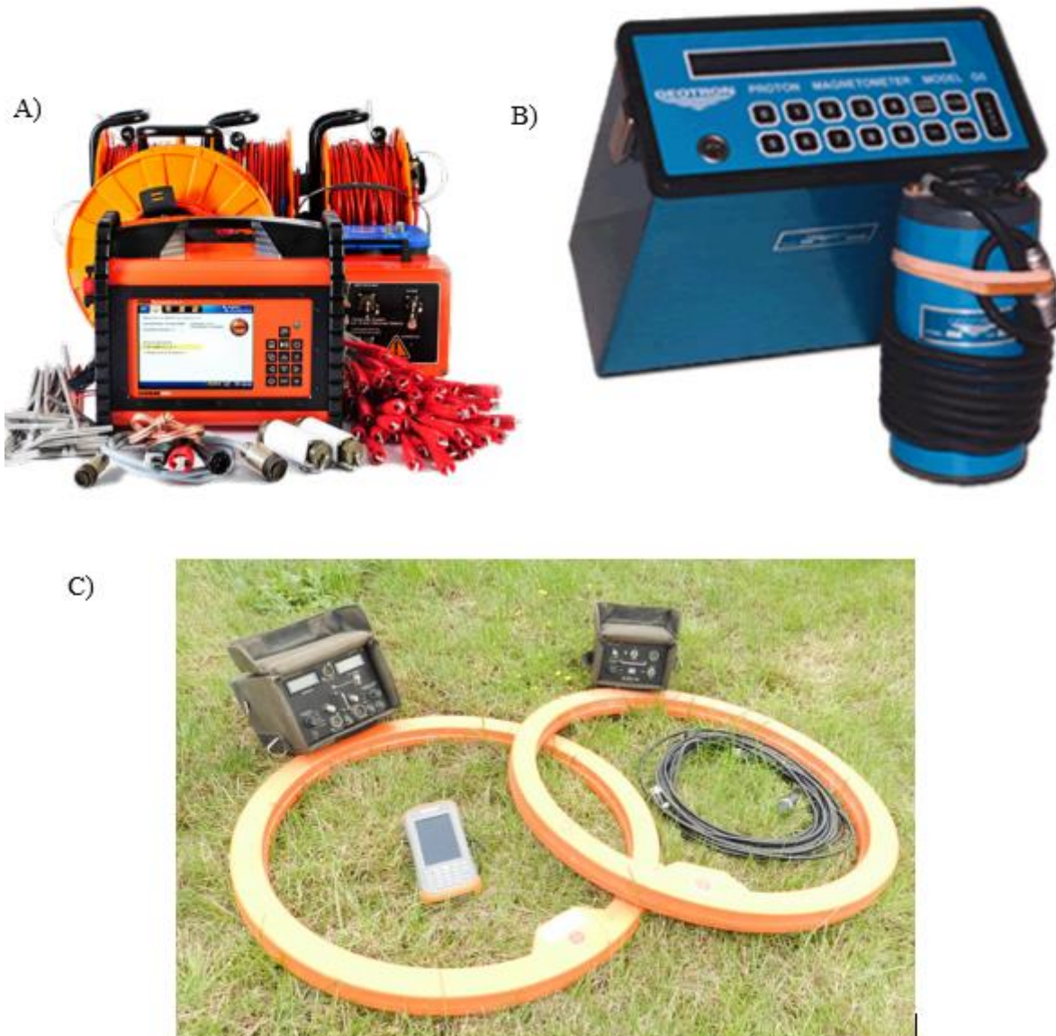
Figure 4.115 A) ABEM Terrameter LS 2 set B) Geotronics G5 Proton Memory Magnetometer C) Geonics EM34-3. Modified from (Guideline Geo, n.d; ASEG, n.d; Geomartix Earth Science Ltd, 2023)
