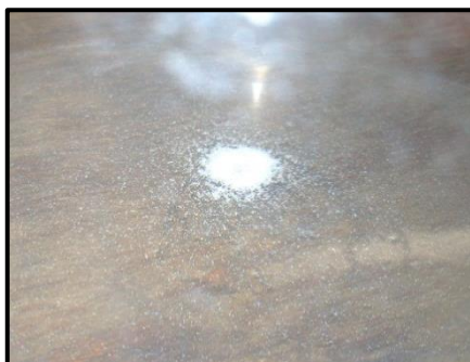
Figure 2.2 A picture showing the low solubility of ZnO in water.
