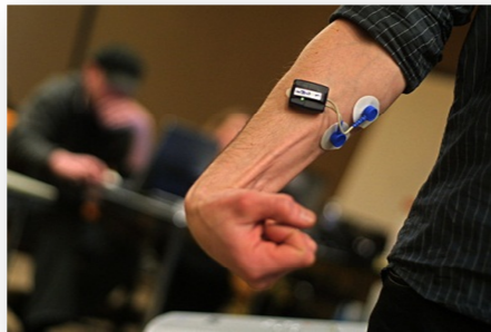
Figure 4: Surface electrodes measure electric currents in muscles (Search Directories.com, n.d.)
