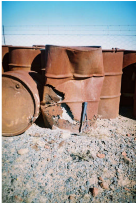
Figure 3.1.9 Rust in 200 litre barrel (no. 3 on location map).
