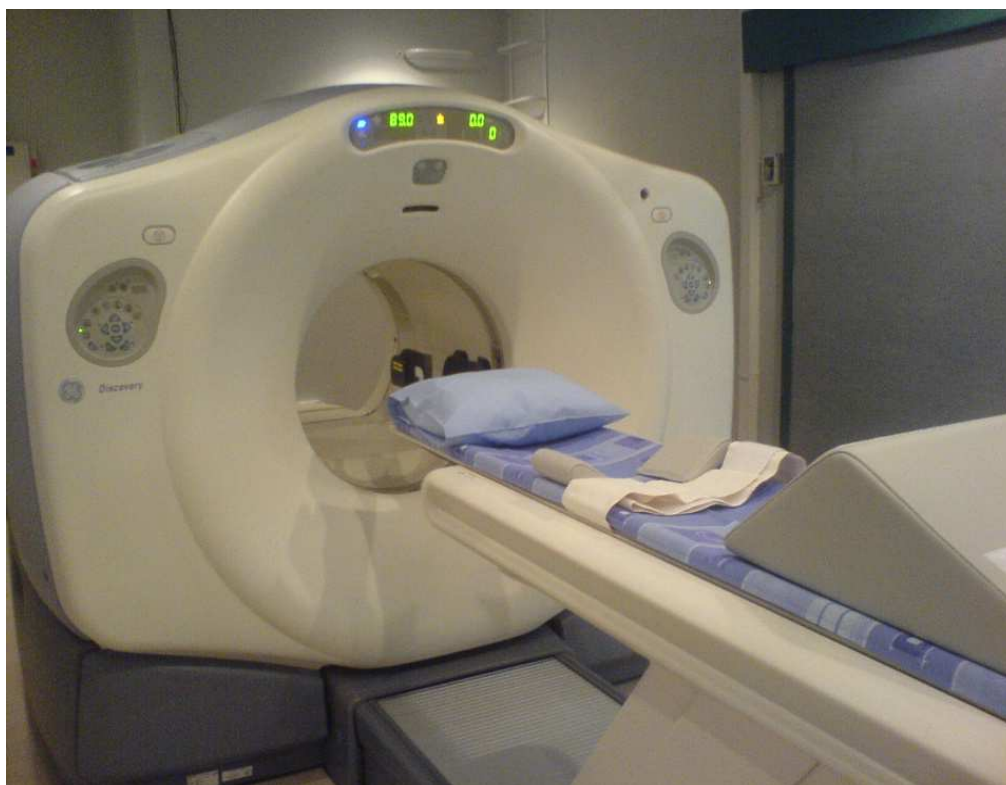
Figure 3-1: GE Discovery ST PET/CT Scanner at the Free State PET/CT Centre that was used for the phantom scans in this research.
