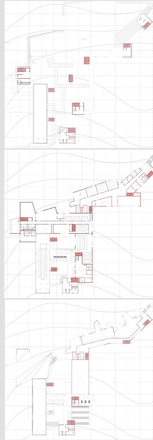
Figure174-176: Left: Core functions, Middle: Serving and served spaces, Right: Fire Escape Staircases (Author, 2022).
