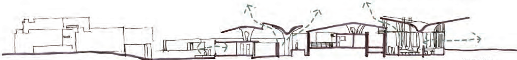
Figure 350: Section showing ventilation
