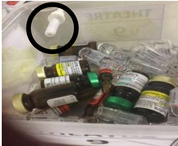
Figure 3: Digital thermometer probe placed within the plastic container containing the drugs
