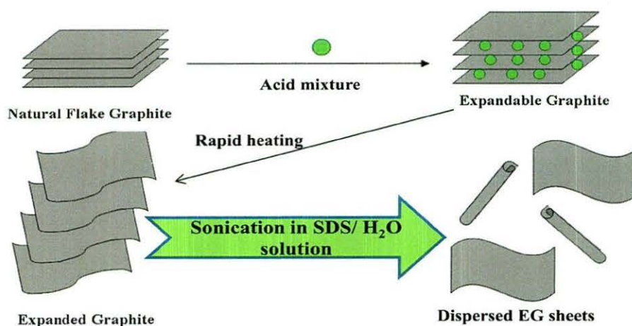
Figure 1.3 Schematic representation of expanded graphite dispersion
