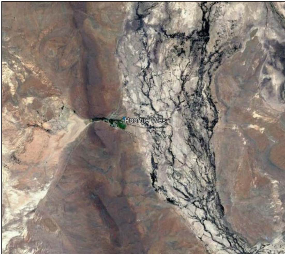
Figure 13: Borehole with potential high yield (12 s \approx 3.9 L/s) in close proximity to dolerite dyke
