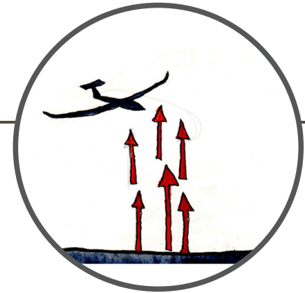
Sketch illustrating thermal lift.
