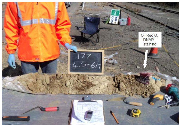
Figure 3-6: Oil Red O ® staining of residual DNAPL in soil boring 177
