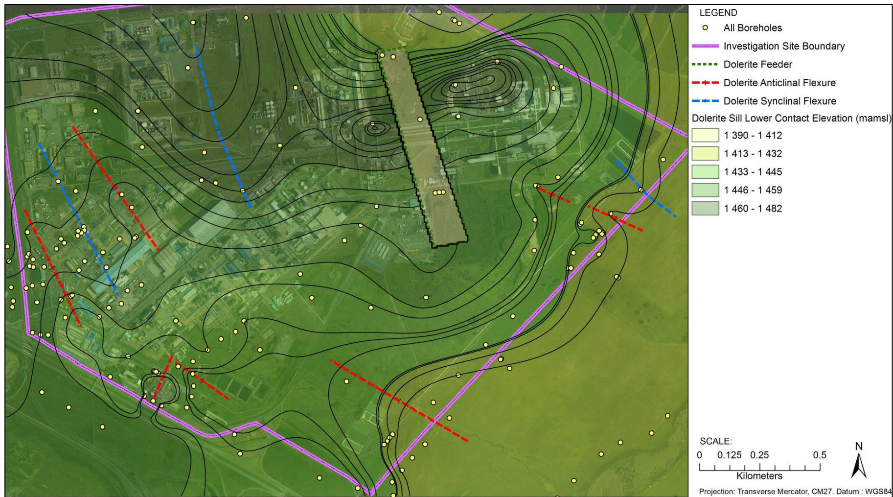
Figure 3-20: Dolerite sill lower contact elevation
