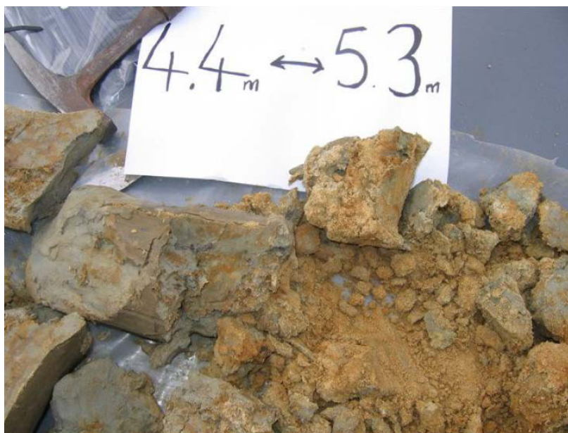
Figure 3-17: Picture taken of roto-sonic core (EDC2S) showing the transition from residual clay dolerite to highly weathered dolerite
