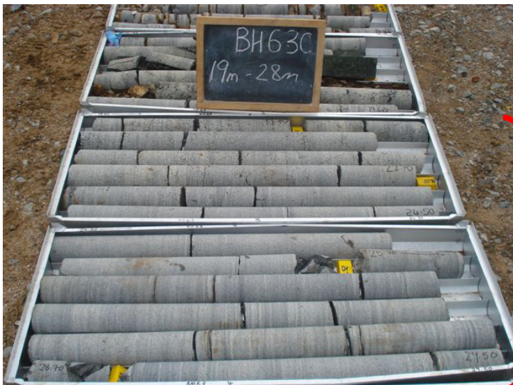
Massive dolerite with low fracture frequency (19-30 mbgl)
