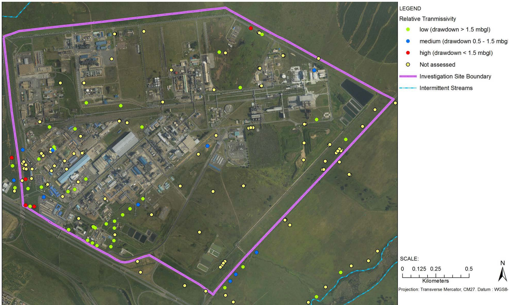
Figure 3-27: Relative transmissivities of boreholes (results from ERM, 2012)
