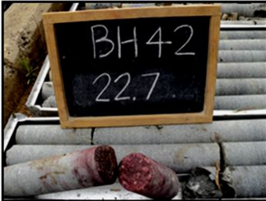
Figure 3-47: Oil Red O ® staining at 22.7 m bgl in core hole CBH42 indicating the presence of residual DNAPL
