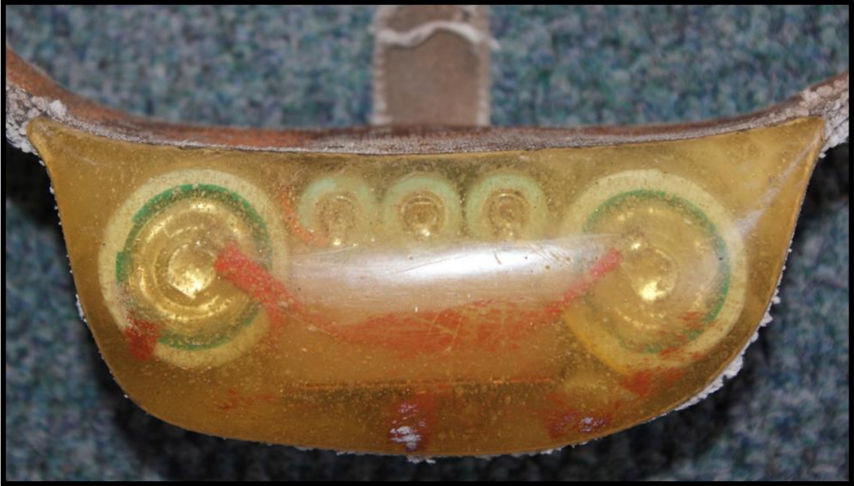
Figure 4.2 Compaction of batteries and VHF monitor transmitter inside the collar
