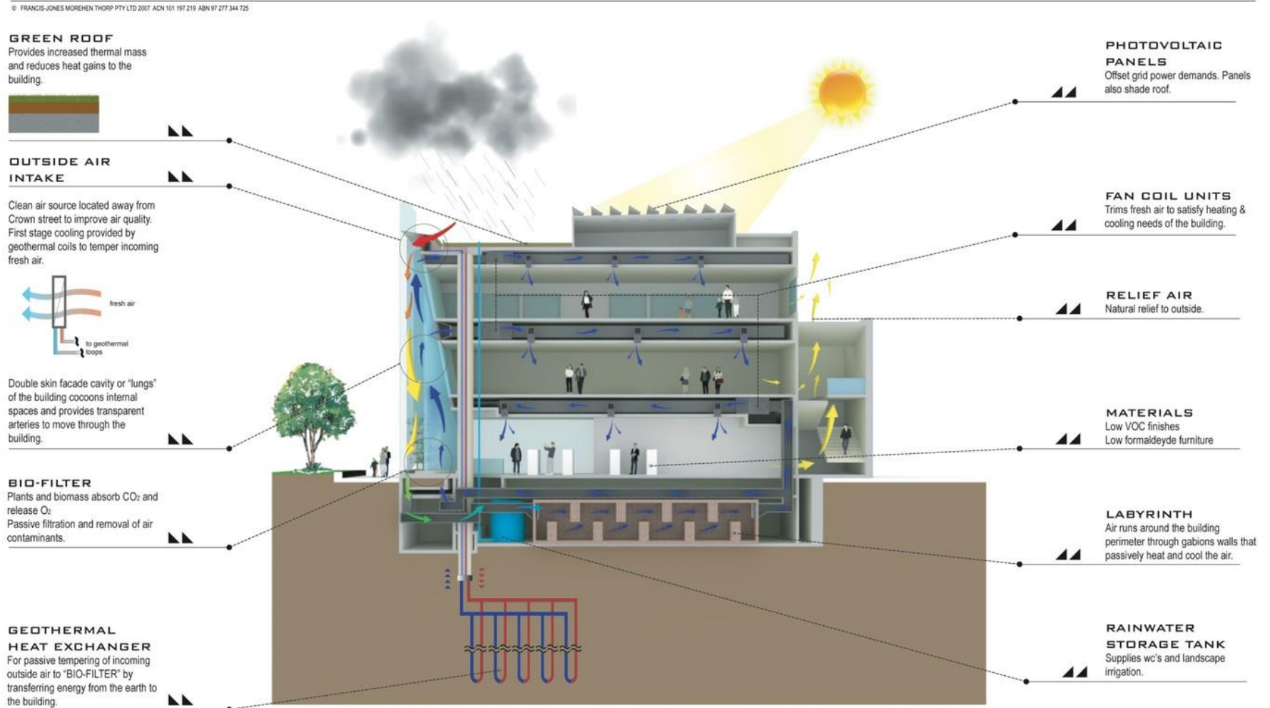
Fig. A Diagrammatic section with annotations of the Surrey Hills Library showing the buildings approach to sustainability. (archdaily, 2009: online).
