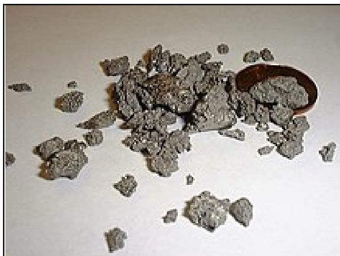
Figure 2.3: Titanium sponge (Stanford materials, 2023)
