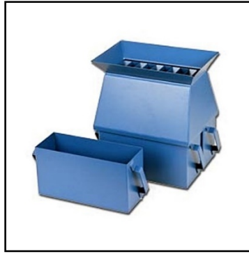
Figure 4.2: Sample splitter (Geology Superstore, 2023)
