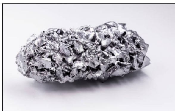
Figure 2.9: Pure titanium metal (Rhj, 2021)
