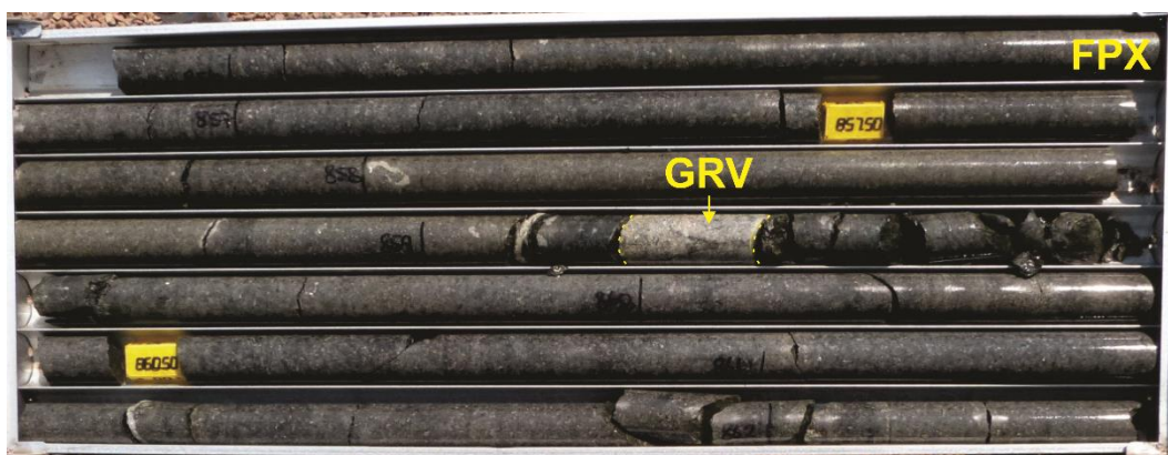
Figure 3.4 Drill core photograph of MD comprising of feldspathic pyroxenite (FPX) with a granitic vein (GRV) cross cutting the lithologies.
