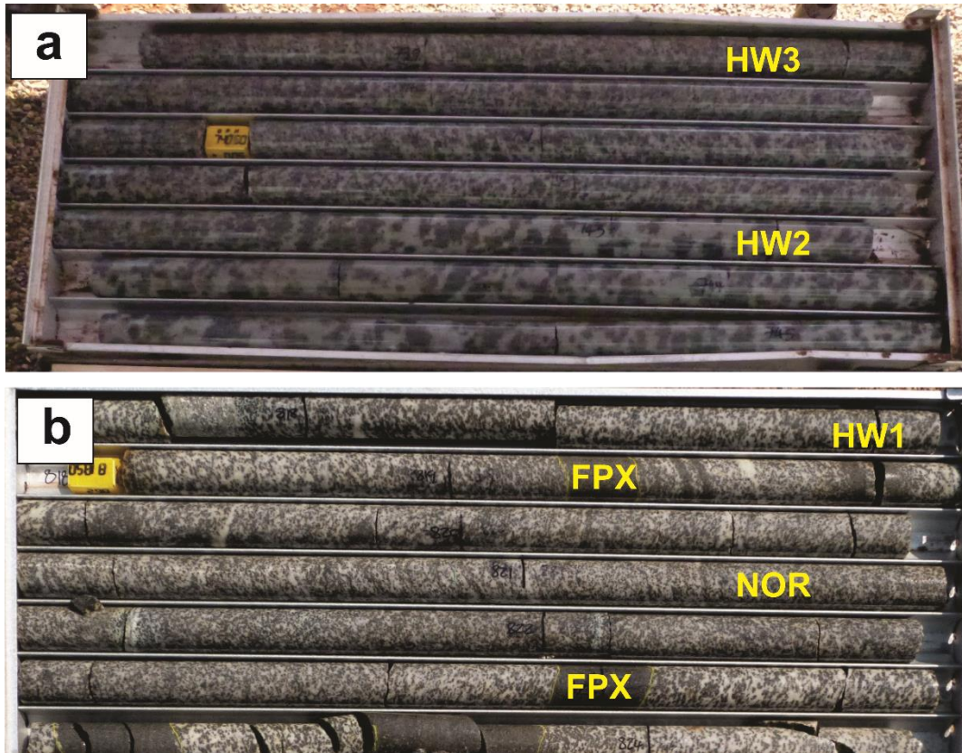
Figure 3.2 Drill core photographs of UMT-393. a MZ norite grades into mottled anorthosite of HW2 that marks the top of the Flatreef, b interlayered norite-pyroxenite at various thicknesses of the HW1. FPX = feldspathic pyroxenite, NOR = norite.
