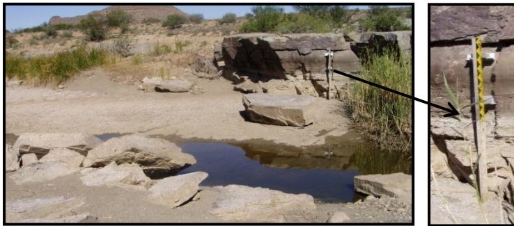
Figure 4.4: The measuring plate at site EWR4 during March 2007, indicating that, although it was dry at the measuring plate there was indeed water in the pool.
