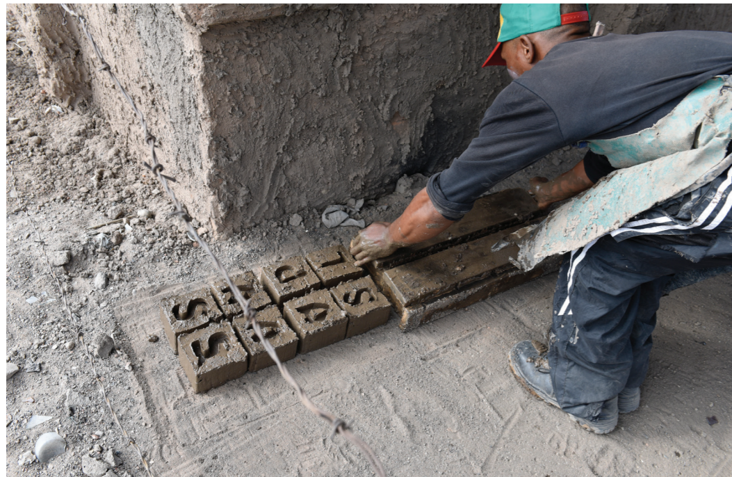
Figure 4.40 Trevor Snyders creating hand-made bricks (Crafford, C., 2016)
