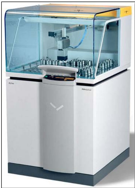
Figure 2.3. The PANalytical WD-XRF Axios spectrometer, Geology Department, University of the Free State.
