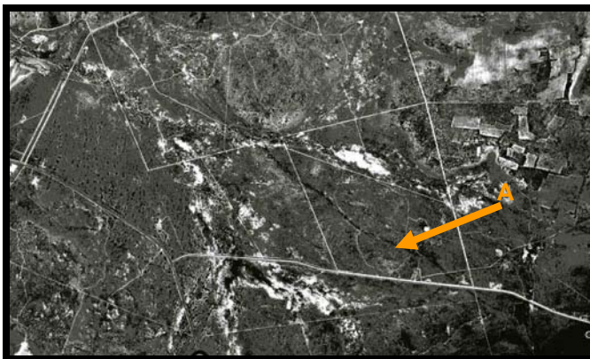
Figure 2.12a. The farm Blokdrift 512KQ (case study 5). A diabase intrusion demarcated by linear, dense vegetation growth (A) (darker texture).
