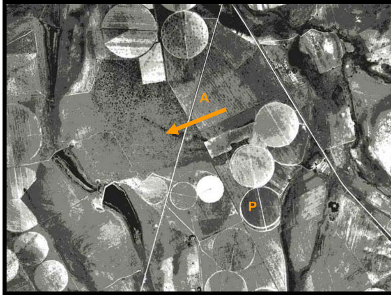
Figure 2.12b. The farm Hartbeesfontein 394KR (case study 30). Linear, moist (dark texture) patterns due to a lineament (A) in the Bushveld that are even manifested on the circular irrigation-pivot lands (P).
