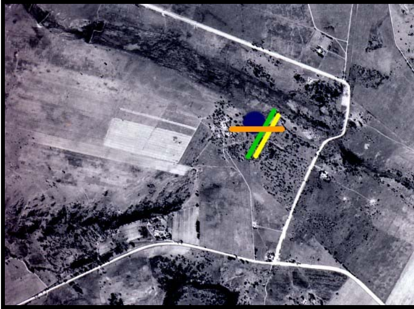
Figure A1.29. The geology (top left, Figure A1.28), land type (top right, Figure A1.28) and aerial photograph of Zusterstroom 447JR. The blue circle denotes the position of the borehole, the green line the orientation of the magnetic profile, the yellow line indicates the electromagnetic profile and the orange line the direction of the Schlumberger sounding. The area covered by the aerial photograph is indicated by the left purple shape in the geological map (Figure A1.28).
