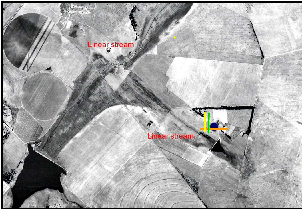
Figure A1.36. Aerial photograph of Trigaardspoor 451JR. The blue circle denotes the position of the borehole, the green line the direction of the magnetic profile, the yellow line the direction of the electromagnetic travers and the orange line indicates the sounding direction. The area covered by the aerial photograph is indicated by the purple shape and the letter “T” in the geological and land type maps. The geology and land type are depicted in Figure A1.32. Note the linear streams in this geological setting that can indicate the presence of lineaments (weathered diabase).
