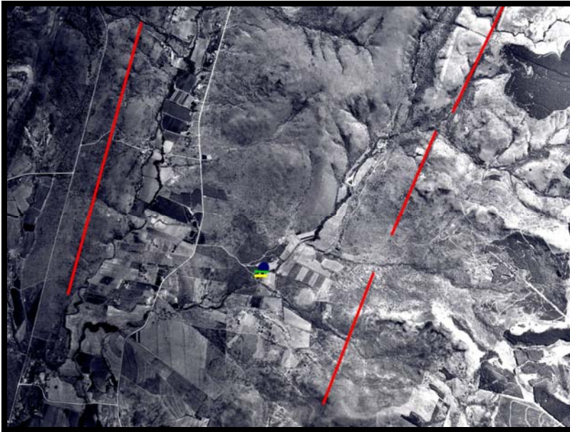
Figure A1.18. Aerial photograph of Rietfontein 88JT. The blue circle denotes the position of the borehole, the green line the direction of the magnetic profile and the yellow line indicates the electromagnetic travers direction. The area covered by the aerial photograph is indicated by the purple shape in the geological map (upper rectangle). The geology and land type are depicted in Figure A1.16. Red lines indicate lineaments (suspicious linear vegetation growth).
