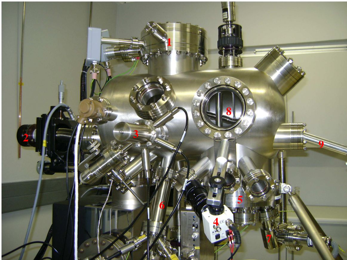
Figure 4.3. The VT-UHV STM system from Omicron at the National Centre for Nano-Structured Materials, CSIR. (1) LEED and Auger optics, (2) Heating manipulator, (3) Sputter gun, (4) CCD camera, (5) STM stage, (6) Effusion cell, (7) LHe cryostat, (8) Viewing window, and (9) Wobble stick.
