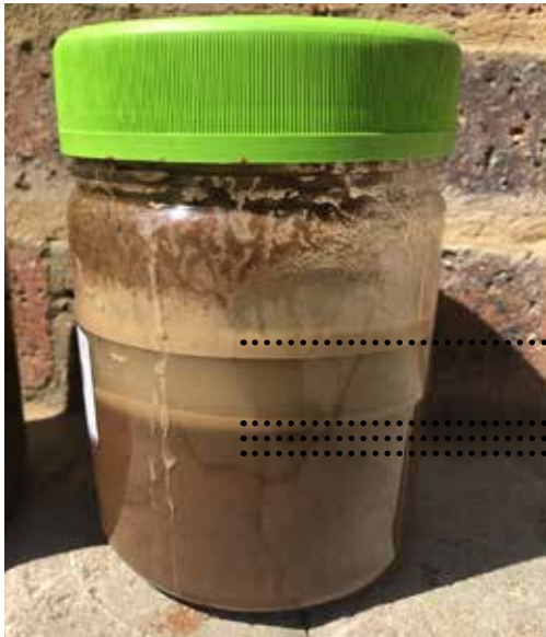
Figure 236: Soil jar test 3: organic matter, clay, silt and sand (Caldeira, 2019: photo).
