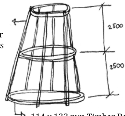
Figure 260: Prefabricated timber pod structure (Caldeira, 2019: drawing).
