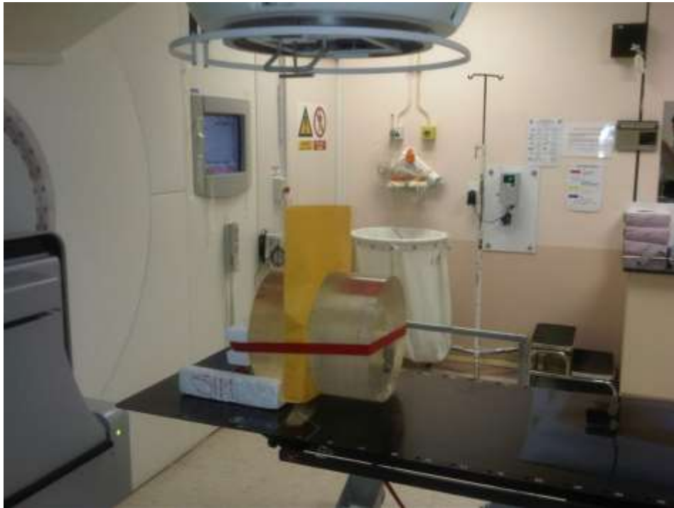
Figure 3.16: The film measurement setup used for determination of dose during image acquisition. An EDR2 film was placed vertically between two perspex phantoms and positioned to coincide with the treatment isocenter. The 200 MU protocol ( -100^{\circ} to 100^{\circ} gantry angle, 1\text{ MU/degree} ) was used to irradiate the film.
