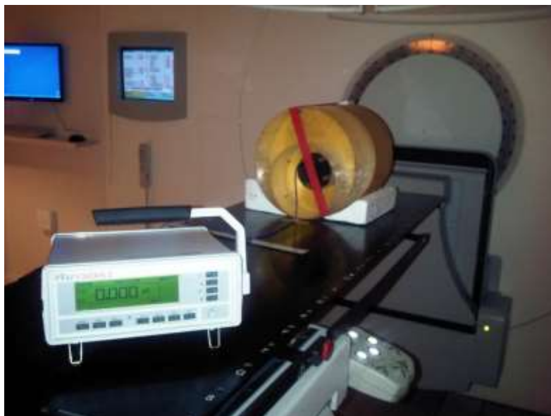
Figure 3.15 The ionization chamber and electrometer setup used to determine the dose delivered during the image acquisition process. The ionization chamber was placed in the center of a cylindrical perspex phantom such that the active volume coincides with the treatment isocenter.
