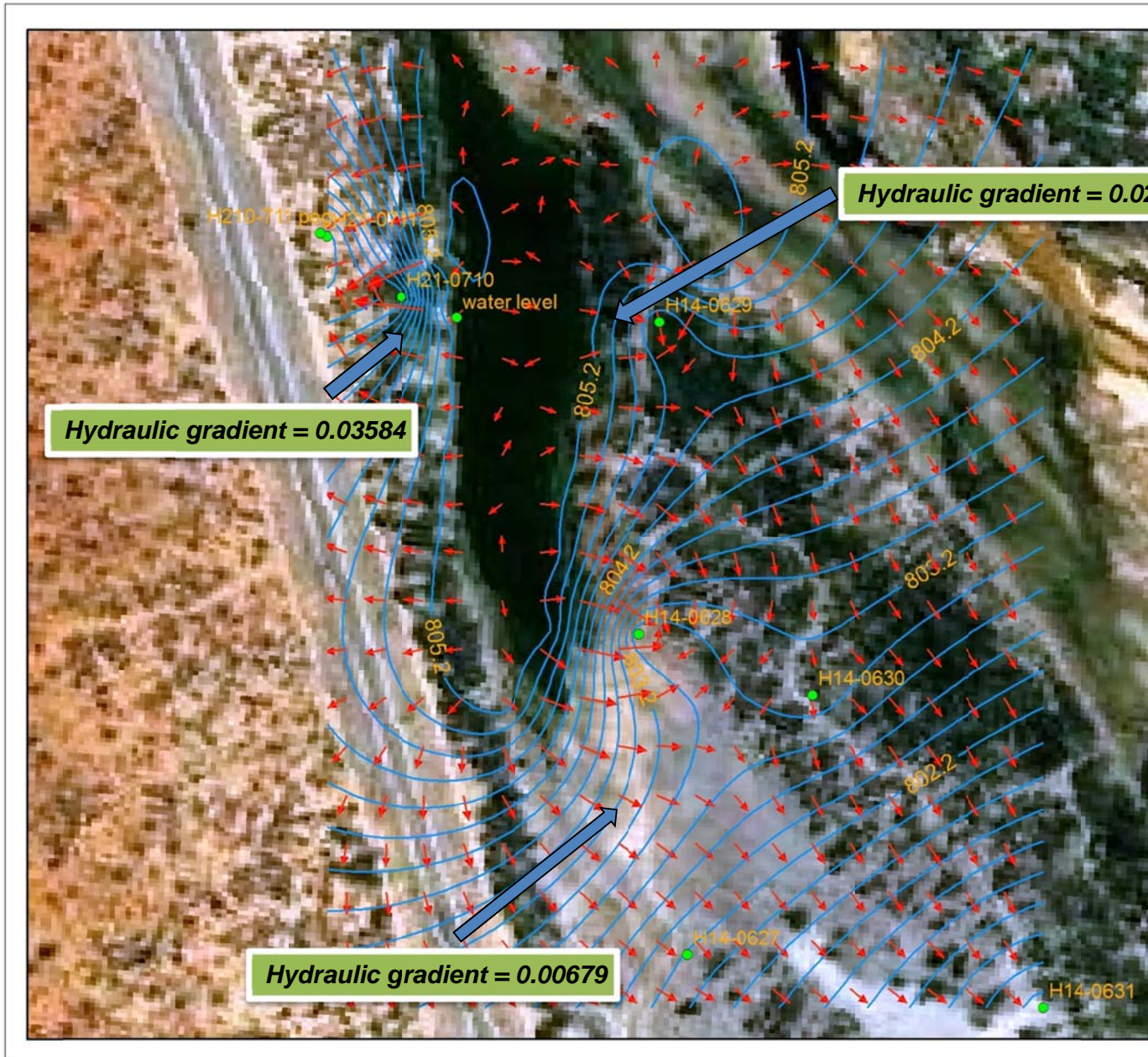
Figure 79: Groundwater flow vectors indicating flow in the vicinity of the Shot Belt Pool (Department of WaterAffairs 2 , South Africa, 2010)
